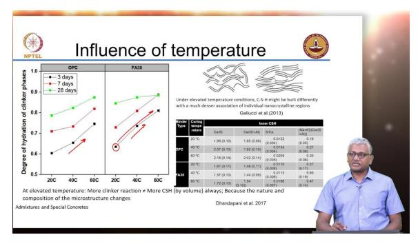
Again this is an example of the degree of hydration that happens at higher temperatures. So again you see that as you increase the temperature the degree of hydration of clinker phases increases and with fly ash again you see that the degree of hydration of clinker phases  $C_3S$ ,  $C_2S$  etc is quite high and increases significantly as you increase the temperature.
