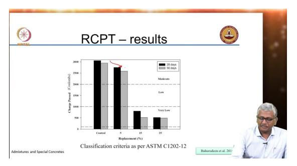
So in RCPT again for 5% replacement you do not see a major drop but at 15 and 25% your RCPT charge passed is falling to very low values less than 1000 Coulombs.
