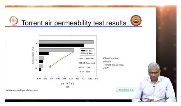
We also did another air permeability test on this concrete. This was based on an apparatus that is available for field testing. So this air permeability test method can be also applied to concrete in the field and again you see very clearly as you increase the level of replacement the permeability coefficient as measured by this test is coming down significantly. You see a major drop in permeability coefficient and of course the greater your cure the greater the drop.
