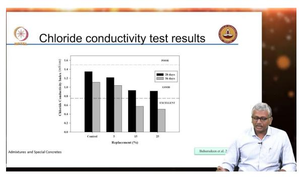
Chloride conductivity again you are producing much lower conductive concrete with respect to chlorides.
