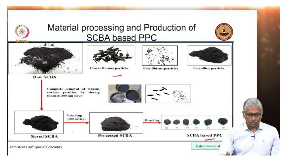
So as I said sieving to remove the fibrous particles and then grinding to cement size was used to actually produce the Portland pozzolan cement of which the properties I have already shown you previously.
