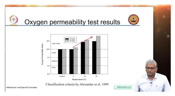
Oxygen permeability again your result here clearly this shows that with increasing levels of replacement, you are producing a concrete which is less permeable to gases. Of course qualitatively the performance of all concretes is a very good category.
