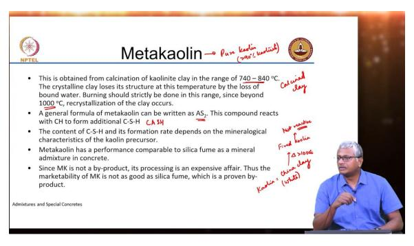
You cannot go with high replacement levels when you are looking at carbonation resistance. So let us move on from fly ash to slag to metakaolin. Metakaolin is the name given to calcined kaolinite clay, calcination of kaolinite in the range of 740 to 840 degrees Celsius. What is kaolinite also known as? What is the common term for kaolinite? Market term? It is China clay. And where do we use China clay? For ceramic, for paints, all of these are applications.
