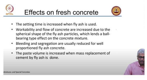
Now fly ash reacts slowly, so setting time is going to increase. Workability and flow of concrete are expected to be increased because of the spherical nature of the fly ash particles and just like air voids, the spherical nature of fly ash particles lends a ball bearing type effect that increases the flow ability of the system.
