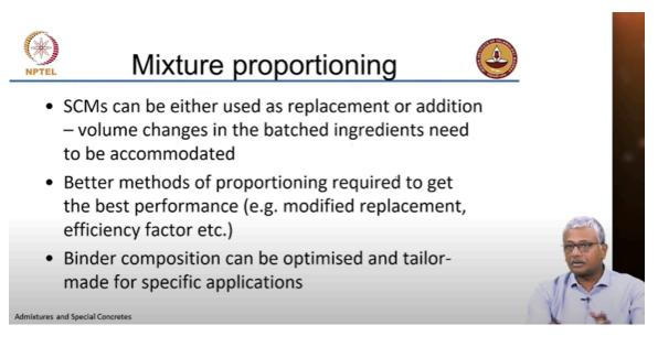
So in conclusion with respect to the activity testing of materials it is very important for us to judge the extent of reactivity shown by any mineral additive or supplementary material before we start using it in concrete. We cannot really take a material which is newly created and start putting it as a replacement of cement in concrete without assessing what
