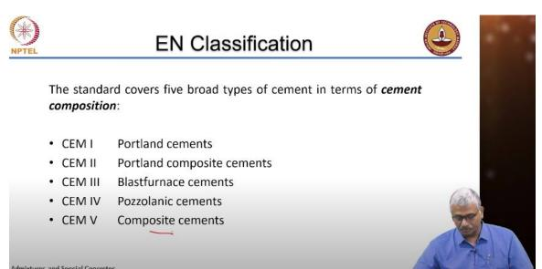
Again similar but EN has a much more diverse classification of cements. So they talk about CEM 1, 2, 3, 4 and 5 where they talk about Portland cements, composite cements, blast furnace cements, pozzolanic cements and they have composite cements which have much larger levels of substitution.
