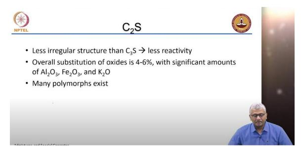
$C_2S$  is a less irregular structure that is more rounded as we saw from the pictures of the cement clinker that I showed earlier and because of this more regular structure it has got less reactivity. Over all substitutions of oxides can be up to 4 to 6%. So in belite  $C_2S$  can have impurities in the form of these oxides and again because of the formation and the presence of different types of impurities the polymorphs exist.
