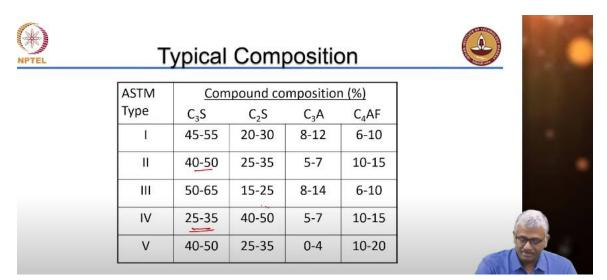
So this is the overall chemical composition which is quite similar if you look at the other standards like BIS, It also has a sulphate resistant cement, BIS also has low heat cement, high early strength cement, most of the characteristics are quite similar across different standards.
