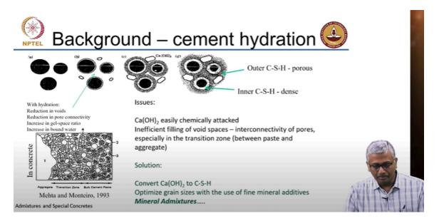
Now we talked briefly about cement hydration in the first segment of this course. The idea is that as hydration proceeds the porosity gradually fills up with the products of hydration. What are these products? Calcium hydroxide and ettringite and probably later monosulphate and other calcium aluminate hydrates. As the filling up of the porosity
