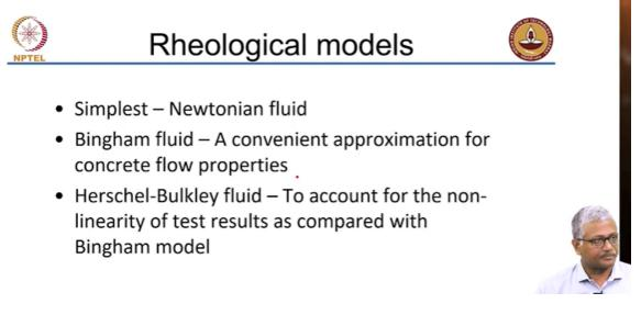
So most materials are described by their rheological behavior and this behavior can be captured with the help of simple models. The Newtonian fluid model is the simplest model which applies to water or oil. As soon as they start shearing the plates, the water will flow. Any shear that is applied will cause the water to flow.
