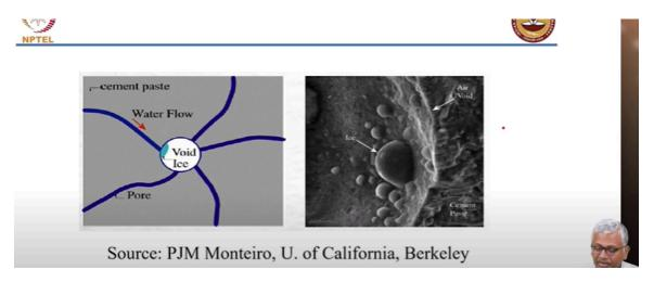
So again this is again a picture from University of California Berkeley where very nicely they are showing the formation of ice in the walls of a void, air void. What is the difference between a void and a pore? Voids are usually discrete. Pores are more or less continuous channels through which your water is flowing.
