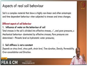
So, stepping into the real aspects of soil behaviour aspects of real soil behaviour soil is basically a complex material that shows a highly non-linear and often anisotropic and time dependent behaviour when subjected to stresses and stress changes. So, usually these stresses keep changing day by day or after t = 0 or t = 1 or t = n. The stresses are not all constant, they are changing, they are changing you know with time.
