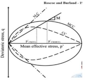
So, this is your original cam clay model failure locus and this is the failure locus of here modified cam clay and I have also put for your reference this is the value locus that you obtained for Mohr Coulomb model so it keeps expanding. So, this is the failure locus you generally observe in case of a modified cam clay model using this particular failure equation.
