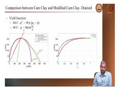
So, here I am trying to compare the stress strain and volume change response between the original cam clay model and the modified cam clay model. As you can see the failure locus somewhat leaf-like because of the presence of logarithmic term in case of original cam clay model and this is an elliptical failure locus in case of an modified cam clay model. This is your failure line failure and M.
