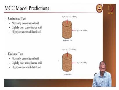
Once you have all these things we can actually model and try to predict the material response. So, this is a typical response what you observe in an undrained and drained condition. When you are performing a normally consolidated soil and when you are having a lightly over consolidated and highly over consolidated soil.
