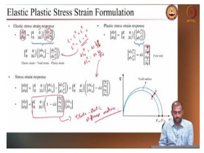
So, this is your basic yield function. Using this yield equation and the plasticity framework which we discussed how do we model the material response. We will see with some examples we will see how using this model we can predict both trained and undrained response. So, as we know this is an elastic stiffness matrix. So, the volumetric part the mean effective stress and the deviatoric stress are related to the volumetric strain and shear strain using the stiffness matrix.
