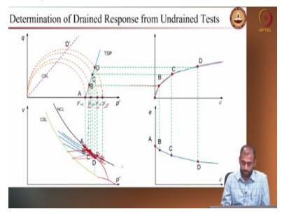
So, you have this new pre-consolidation pressures. From this you can actually draw the stress profile for the drain test. So, you already know the undrained behaviour but you are trying to predict the drained response. Also, the challenges since you it is undrained interest you have only the pore pressure response but you want to know the volume change response if there is an undrained test that has been performed.
