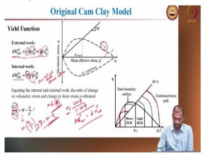
Based on these results they proposed the yield function. So, as I said this is based on energy principles. So, what they did is they tried to write the external work. So, this is external work is nothing but the mean effective stress that you are applying and the corresponding plastic volumetric strain increment and the deviated stress you are applying in the corresponding D matrix strain increment.
