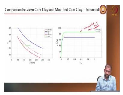
And the pore pressure is sort of overpriced in case of OCC. So, as we saw the limitations we actually try to predict and then we showed that the stress strain response between OCC and MCC.
