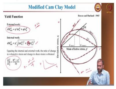
To avoid this in 1965 Roscoe and Burland came up with a modified version of this cam clay model. So, what they did? They use the same external work similar to the original cam clay but they modified the internal work. So, still they use the internal work M so the material property M in addition to that they slightly modified the internal work equation. Modifying this resulted in a dilatancy equation which is not linear.
