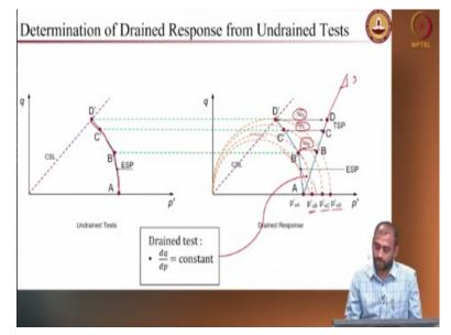
So, one of the advantages of using these models is that you can use the critical state framework, you can use this model and if you just have a drained response or if you have an untrained test but if you want to quantify the drained response you can use this framework and quantify the drained response from the undrained test. So, for example this is your undrained test so this is between p prime q space you are having in this sort of an undrained response.
