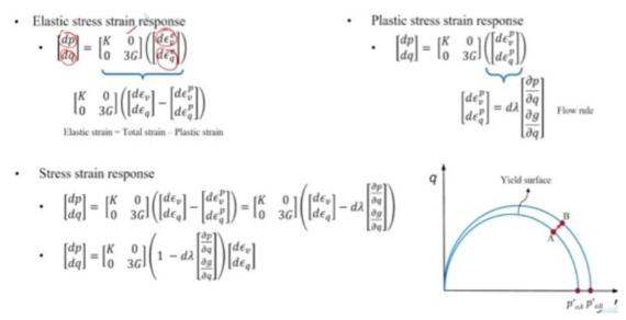
So, we all know total strain is equal to elastic strain plus plastic strain. So, if you want to know the elastic strain is equal to total strain minus plastic strain. So, if you just write this in this equation and we have the relation for the plastic strain. Plastic strain d epsilon v p is nothing but d lambda into dp by dq sorry I think this is there is a error here. So, this is dg by dp. Similarly, d epsilon qp = d lambda into f by dot q.
