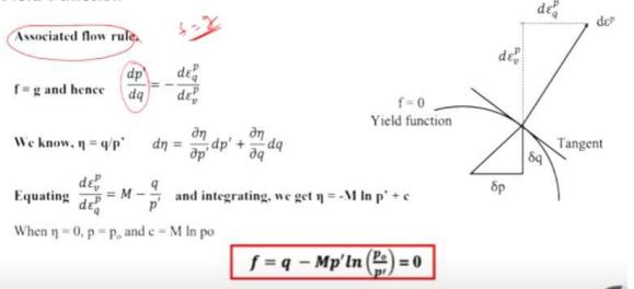
This is a function of p 0 this the pre consolidation pressure so you have this particular p 0. So, you have this particular failure equation. So, since it has a logarithmic term in it the shape is like a log spiral or not a log spiral, I think the shape is like a leaf-like shape which is a logarithmic
