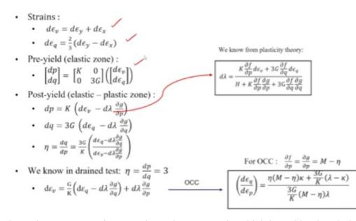
So, you have these two equations you have the stress ratio which is nothing but dq by dp prime. So, in case of drained test so your eta = 3 this is always the stress path is always taking in a slope of 3. So, you can use this condition to derive your volumetric strain response. So, again we use an associated flow rule so you use M - eta and then try to form the equations. This is the formulation for drained response.
