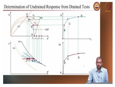
So, you can find out the difference between the total stress path and effective stress path to find to plot the pore pressure curve. Similarly, you can also apply identify the specific volume in this particular space. So, you have a drained test and you are trying to predict the undrained response. So, this model this original cam clay and modified cam clay model predicts the material response fairly accurately.
