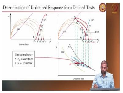
Similarly, if you have drain test and if you want to determine the undrained response. So, if you have a drained test, you will have this particular total stress path of a slope three. So, once you know this how to determine the untrained response. So, you know the pre-consolidation so from the Mohr Coulomb failure envelope you will determine PC POB which is the pre-consolidation pressure at the point B, point C and point D.
