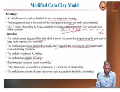
So, again as I said this has an advantage. So, it is a unified framework which predicts both the shear and volume change behaviour fairly accurately. And the input parameters are few so you can actually perform some triaxial compression test and obtain the model parameters, triaxial
