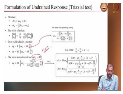
So, for that again as I said we know the volumetric strain, we know the deviatoric strain, preyield you have only the elastic stress strained relations. So, this K and g is just constant but you can make it as a function of sigma 3. We can use pressure dependent bulk modulus and shear modulus and post yield you can also you will also have you will follow the elastic plastic stress strain relations.
