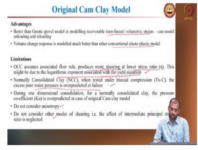
So, because of this I think the shearing response is different. So, what actually the problems since it is having a logarithmic term. So, this might be due to the logarithmic exponent associated with the yield equation. So, it produces more shear stress at lower stress ratio. So, since it produces more shear stress at lower stress ratio it is sort of over predicts then so that is avoided using when you start using a modified cam clay model. So, these are some of the limitations.
