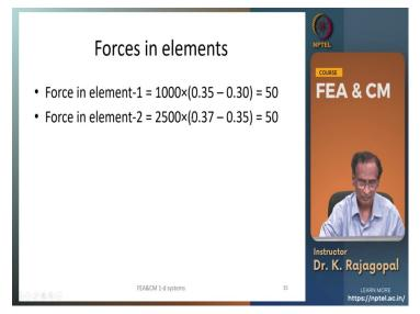
And that is what we want to do 3 is a fixed as a 0.3 and the force in element 1 is 1000 times u 3 - u 2 that is the relative deformation that is that comes out as 50. and the force in element 2 is 2500 multiplied by 0.37 - 0.35 and that comes to once again 50 because they are in in series.
