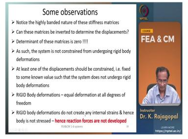
So, the first thing that we need to notice is that the stiffness Matrix is highly banded and most of the elements are zero meets column. So, if you apply a Gauss elimination procedure for this system we just need to eliminate one value below the diagonal in each of these columns. So, it becomes very simple but then if you have to invert this Matrix you need to spend a lot of time and the determinant of these matrices is also zero.
