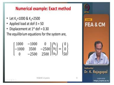
Now let us look at one numerical example so, that we can give some values and then understand the calculations better let us say in this previous example of 2 elements with the spring 1 K 1 and spring 2 K 2 we applied a load of 50 a degree of freedom 3 and a degree of freedom 1 we constrained the displacement to point three the server equilibrium equations are like this see this K 1 is thousand and K 2 is 2500.
