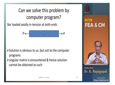
So, let us look at conceptually very simple problem. Let us take one axial element and then go on pulling at the 2 sides by an equal amount. And we know that this system is in equilibrium because we have applied equal and opposite forces at the 2 ends. And the solution is obvious to us the axial force is equal to P that is the tensile force and the stress is P by Del P by A.
