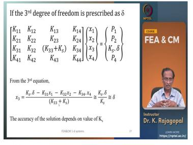
So, on the same problem say we are constraining the third degree of freedom to sum Delta and we can add the KS to the diagonal element of this stiffness Matrix and then on the right hand side we can apply a force equal to KS times Delta and this K is so, large that compared to all the other forces that are developed the K 31 times x 1 K 32 times x 2 K 34 times x 4 they are very small and negligible.
