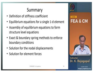
Just to summarize in this lecture we have defined the stiffness coefficient for a one dimensional element. Then we form the equations for one for a single element then assemble them for multiple elements and then we we have seen how to apply the boundary constraints either by exact method or by the boundary spring method and then we can once we apply this boundary constraints we can solve the equations then we got the solution for nodal displacements and then the element forces.
