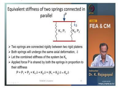
And let us consider that 2 elements K 1 and sorry element one and element 2 are connected rigidly between 2 patterns and the stiffness of element one is K 1 and stiffness of element 2 is K 2.
