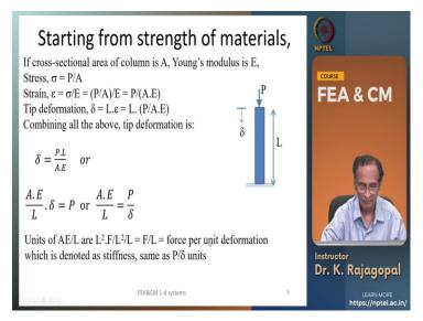
So, let us start from the most fundamental strength of materials because all of us are familiar with this famous equation Delta is equal to PL by AE that is the the equation that we study the first thing in any of the strength of materials courses.
