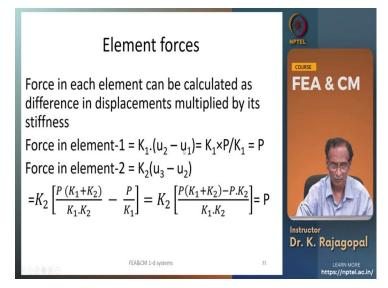
And once we get the deformations we can find the forces in the 2 elements the force in element one is a K 1 times u 2 - u 1.
