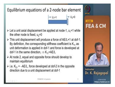
So, let us apply unit deformations in different directions and then measure the forces. So, that we can define our stiffness coefficients K ij and to start with let us apply a unit deformation a degree of freedom 1 that is u 1 is equal to 1. And while we are doing that we constrain this node or this degrees degree of freedom u 2 to 0. And so, the unit deformation at 1 will produce a force equal to A E by L times 1.
