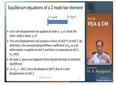
And similarly we can apply a unit displacement at a degree of freedom 2 while we constrain this degree of freedom from moving. So, by doing this we can write that K 22 is a by L that is the force developed in degree of freedom 2 because of a unit displacement a degree of freedom 2. And the force developed at degree of freedom 1 because of a unit displacement a degree of freedom 2 will be K 12 and that should be equal to - AE by L to maintain our equilibrium.
