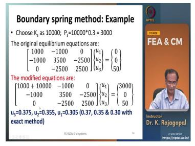
And let us look at the boundary string method to illustrate and let us take the boundary spring stiffness is ten thousand. So, the PS is a three thousand one thousand ten thousand times point three it is our original equations are like this
