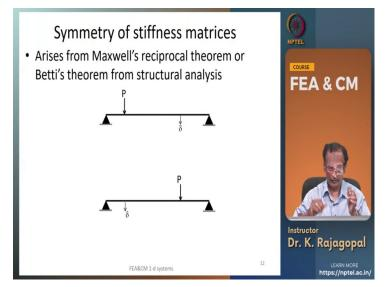
And now see we see that our system of equations gives us symmetric stiffness Matrix. See K 12 and K 21 are the same - AE by L and this symmetry we can imagine by looking at the reciprocal theorem Maxwell reciprocal theorem.
