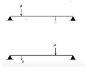
That is so, if we have a structure with a load applied at one point and you measure the displacement at some other point or apply the load at the other point and measure the displacement at this point the Delta should be the same.
