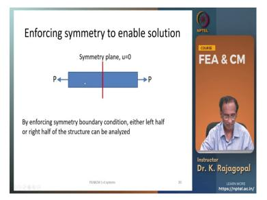
So, the Symmetry plane our displacement is zero. So, this is what we can enforce on the system that at this point my displacement is 0 and then you apply the force and then find the deformations. And once we apply this you know deformation constraint on the Symmetry plane then we can either solve the right hand side the half of the problem or the left hand side it does not matter because both will give the same result.
