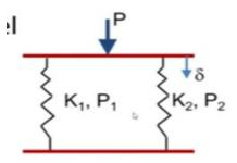
And when we apply any Force both will undergo the same deformation because they are connected with the rigid pattern the same displacement Delta in both the elements. And let us say that the combined stiffness is KS that is the contribution from element 1 and contribution from element 2.
