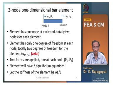
And let us start with one dimensional bar element that is purely axial all the deformations are only in the axial Direction and also the forces are in the axial Direction either tension or compression.
