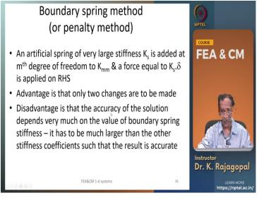
And so, we should have some other method for applying a similar constraints and that is called as a boundary spring method. And so it is also called as a penalty method because on the system we apply some penalty so, that we can enforce what we want. And what we do is we take an artificially an artificial spring of very very large stiffness case and add it at the empty degree of freedom where we want to apply some constraint and then apply a force equal to KS times Delta on the right hand side.
