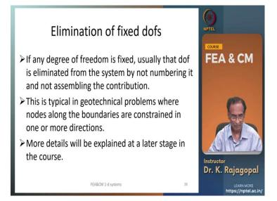
So, now by doing one of these methods we can we can enforce the constraint or the other method is if any of the fixed degrees of freedom is there we can directly eliminate that right from the beginning and we do not number that particular degree of freedom and assign any stiffness coefficient. And especially this is typical of geotechnical problems where we have very very long boundaries where our displacements are zero.
