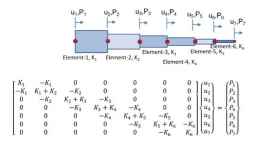
And these are the displacements u 1 u 2 u3 u4 u for u 6 u 7 and then these are the applied forces and um the determinant of this bigger Matrix is also zero that we do not need to doubt.
