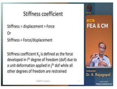
So, this stiffness coefficient is required because we require to calculate the reaction force that is calculated as stiffness times displacement and that is equal to the applied force on the right hand side. The stiffness is a force divided by the displacement and in general we Define stiffness coefficient K ij is actually we are going to deal with the multi degree of freedom system.
