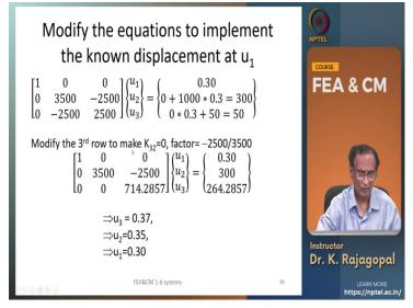
And our known quantities we can take to the right hand side and here it was - 1000. So, - 1000 times 0.3 if you send it to the right hand side we get 1000 times 0.3 that is 300 and then at the degree of freedom 3 we have applied a force of 50 and we can solve this by converting this to an upper diagonal matrix and we get the u 3 as 0.37 u 2 is 0.35 and u 1 is 0.3.
