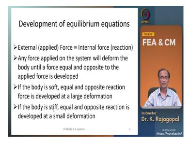
And so, what we mean by the equilibrium is externally applied force should be exactly equal to the internal force of the reaction that is a reaction is developed by the body to resist the applied forces. And so, any force that we apply on the system will produce some deformations that we may be able to measure with a ruler or with a micrometer or something depending on the magnitude of these deformations.
