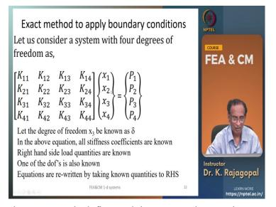
Let us look at the exact method first and let us say that we have a system of four simultaneous equations with four unknowns  $x \ 1 \ x \ 2 \ x \ 3 \ x \ 4$  and then the applied forces are P1 P 2 P 3 P 4 and let us say that one of these degrees of freedom x 3 is known to us or it is constrained to be Delta and after solving our Delta x 3 should be equal to Delta. And in here if we see these are all the known quantities K 11 K 12 K 13 and so on.
