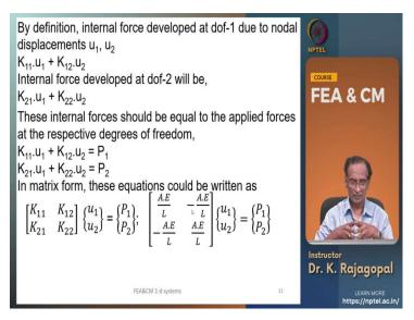
So, by combining these the internal forces developed can be written like this the internal Force developed a degree of freedom 1 because of displacements u 1 and u 2 will be
