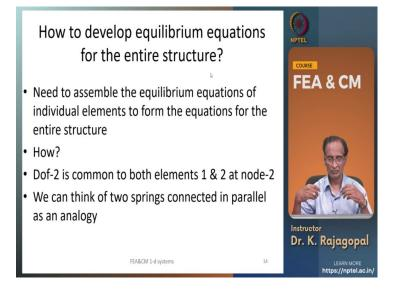
And now we have to see how we can develop the equilibrium equations for the entire structure. See now we have determined the equilibrium equations at the element level at for element 1 and element 2 separately. And we need to form the equilibrium equations for the entire structure and that we can do by assembling assembly of the contributions from different elements. And so, if we assemble we get the equations for the entire structure but how.
