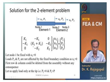
And so, here let us go back to our 2 element problem and let us say that our u 1 is 0 and P 2 and P 3 are not affected because our u 1 is zero. So, it is the first row and first column can be can be eliminated because the P 1 is is not affected because this displacement is zero. And so, we can eliminate the first row and the first column and we end up with a 2 by 2 Matrix like this.
