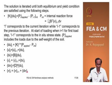
So, the analysis proceeds like this K multiplied by d u i is P i that is the applied - P i - 1 internal and P i is the applied force like, for example, our stress that we applied and the internal reaction that is because of the stresses that are allowable within the material and the integral B transpose sigma i - 1 is your P i - 1 and so as we repeat the analysis our out of balance stress will go on decreasing.
