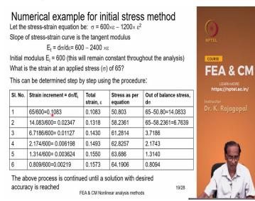
So, now let us apply this to a simple equation because I am going to demonstrate all these through simple hand calculations because if you do through finite element programs we will not really know what is happening and let us take a stress-strain equation like this sigma is 600 epsilon - 1200 epsilon square and this is our constitutive equation and the slope of the stress-strain curve is E tangent d sigma by d epsilon that is 600 - 2400 epsilon.
