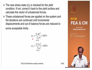
And then once you get this new stress state sigma i we check for the yield condition and if it is not satisfied then we correct it back to the yield surface and then calculate the vector of unbalanced forces and then repeat these calculations until our norm of out of balance forces then the norm of incremental displacements they reach some constant value.
