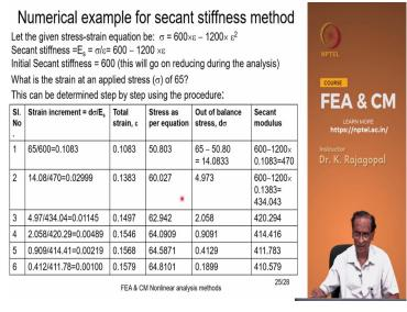
And there is another method called as the secant stiffness method wherein our modulus is the secant modulus is calculated as sigma by epsilon. So, our sigma equation for sigma is 600 epsilon - 1200 epsilon square. So, our secant modulus is sigma by epsilon so that comes to 600 - 1200 epsilon and once again the initial tangent modulus is 600. So, our initial strain increment is 0.1083.
