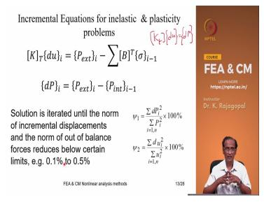
And so we rewrite our equilibrium equations in terms of incremental form, but then our incremental form is written in a slightly different manner K T d u is the applied force P external minus B transpose sigma.
