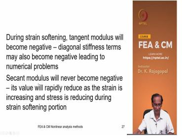
So, the advantage with the secant modulus method is the secant modulus will never become negative. So, we have the ease in the numerical computations.
