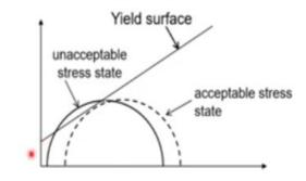
And we have to do something to remove those stresses so that the stress becomes acceptable and so we need to correct the stresses back to the yield surface and so when you correct the stresses back to the yield surface your equilibrium is going to get disturbed. So, in this class of problems we need to satisfy not only the equilibrium, but also certain given yield condition.
