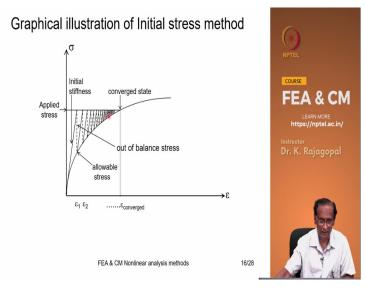
Let us say your stress-strain curve is something like this it is a highly non-linear stress-strain curve and then we have applied a stress of this much and this is the converged state where you are exactly matching with the stress-strain equation and this is your strain at this stress and at our disposal we have only the initial modulus, initial stiffness or initial modulus and the corresponding to that is our initial stiffness equation.
