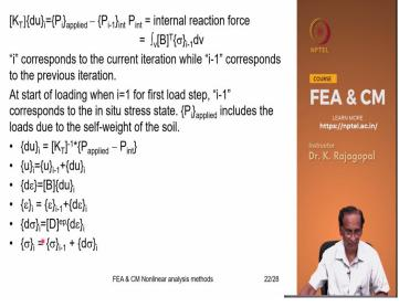
So, the only difference here is we are using this K T instead of K in the initial stress method that K was remaining constant whereas here we are updating it every iteration and every step.
