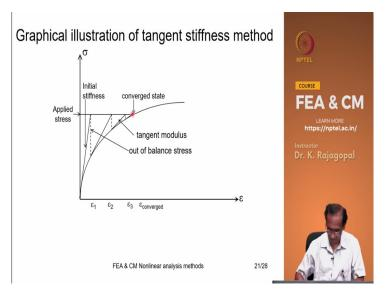
So, let me explain that. So, here we have this non-linear stress-strain equation or the stressstrain curve we applied some stress and we want to know what is the converged strain and so for that we initially apply with the initial modulus. We get some out of balance stress and then we update our stresses and then we get a tangent modulus like this and then once again the tangent modulus at this step this step and so on.
