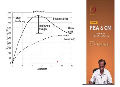
So, even if you are doing this type of strain softening analysis what we do is we calculate at each and every strain softening interval we calculate the secant modulus as the stress divided by the corresponding strain and now let me illustrate this with an excel spreadsheet. I think I forgot to bring my excel file, but I think that we will do in the next class. The first thing that we will do in the next class is I will illustrate the procedure through an excel spreadsheet.
