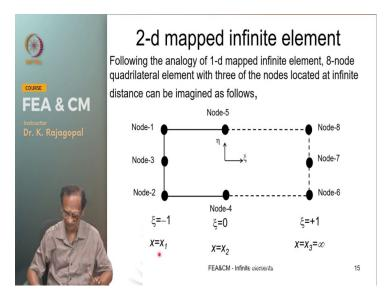
And whatever we derived for one dimensions we can also extend to the 2 dimensions very easily by using our Lagrange method. Let us imagine a night node quadrilateral with the 3 nodes 6 7 and 8 at infinite distance let us define an 8 node quadrilateral like this. Node 1 and node 2 are finitely located and these are the 2 coordinate nodes and nodes 3 4 and 5 these are the mid side nodes at different locations nodes.
