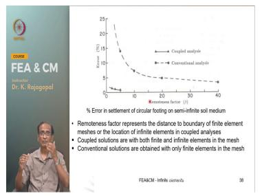
And here is a plot between the remoteness factor that is the distance up to the boundary in the case of finite elements the distance where the infinite elements are coupled with the regular finite elements and on the y axis we have the error. And this line is corresponding to coupled analysis where you have used both finite and the infinite elements and the percentage error is very very small of the order of one percent.
