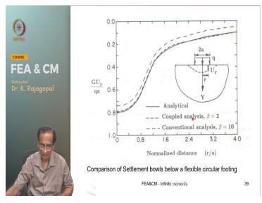
This is the settlement bowl this dark line is the analytical solution and this is our coupled analysis and this is with sorry yeah this is with beta of 2 and this is the conventional analysis with the beta of 10. There is still so, much variation between the theoretical result and then the finite element result when we used our conventional analysis where we fixed the boundaries at 10 times the footing width.
