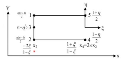
And similarly for getting the mapping function at node 5 we ill use this singular mapping Function One + Xi by 1 - Xi multiply with this to get our mapping function at node 5 you turn it off.
