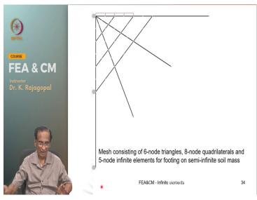
And we can also use combination of quadrilaterals and triangles. So, here drawn some radial lines for representing your infinite distance.
