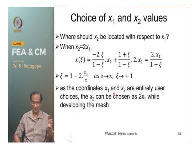
And then another thing that we need to notice is when we had discussed the convergence principles one of the requirements is that our mapping and shape functions should be well defined at all the nodes within the element and but in this case our mapping functions have Singularity at Xi of + 1. So, we are not really satisfying all the requirements of the convergence but then our Sigma of M is g 1.
