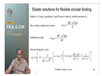
And we can compare our finite element results with the corresponding theory theory of elasticity Solutions. This is the maximum settlement at the center of a bowl center of a flexible circular footing and this is the settlement or the edge of the fitting and these are the stresses along the Z axis Sigma Z then Sigma R Sigma Theta and so on.
