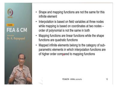
And in this case the shape of mapping functions are not the same we have 2 different sets of functions. See the mapping functions are -2 Xi by 1 - Xi or 1 + Xi by 1 - Xi whereas our shape functions are Xi times Xi - 1 by 2 and 1 - Xi square and so on. Because we are basically 3 nodes for interpolation and the 2 only 2 nodes for the mapping and the 2 for the mapping we have singular mapping functions whereas the interpolation is done by using our conventional interpolation functions.
