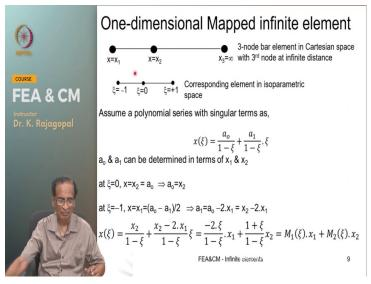
Let us look at one dimensional map infinite element to start with because that is the simplest one. And let us take a 3 node bar element an aXial element with the 2 nodes at some finite distances x 1 and x 2 and let us say the third node is at infinite distance.
