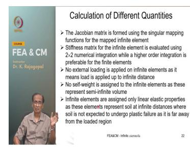
Our Jacobian matrix is formulated using our singular mapping functions. So, when you calculate dou n by dou x dou n by dou Y and so on. We use the mapping functions because we need this dou x by dou Xi dou y by dou Xi and so on. And so, by using the mapping functions of the singular mapping functions we can get our infinity into the calculations then our stiffness Matrix is formulated using our regular numerical Integrations.
