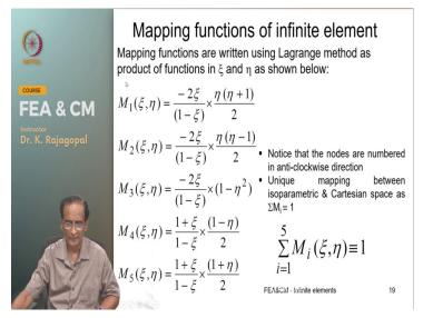
So, by using the Lagrange principle we can get our 5 mapping functions like this and you I want you to notice that we have numbered these nodes in the 90 clockwise direction. Unless you number the nodes in the anti-clockwise direction you will not get your your positive Jacobian matrix or the Jacobian determinant. So, 1 2 3 4 5 and as the convention we numbered the corner nodes first and then the mid side notes later.
