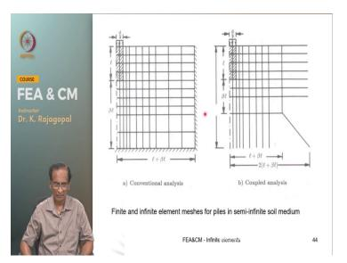
And you can do the same thing even with pile foundations and especially when you have very long pile foundation is hard to decide where you need to keep your boundary because the file length itself is it could be 30 to 40 meters. And beyond that how much soil we need to place either one times 2 times half a time and so on. And so, so in the analysis finite element analysis of piles usually involves in very very huge meshes.
