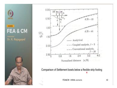
So, here you see the comparison between the analytical and then this finite element Solutions. So, this is for a beta of 2 the D by B comes out about 41 whereas for finite element analysis the D by B is about 12. Although the boundaries fixed at 10 times there is a slight difference it is not coming out exactly as 10 because of the numerical my address.
