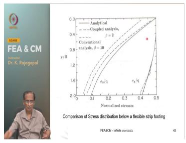
And these are the predicted stresses. The black lines are the analytical stresses and then the dashed lines are from different finite element analysis.
