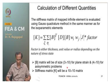
So, how do we do the computations is very simple our stiffness Matrix is written as integral B transpose DB integrated of the volume. And as we had seen with the other Continuum elements we can write the K as a double summation over Xi and Theta B transpose DB multiplied by W i times W J these are the weight factors in the Xi and ea directions multiplied by this determinant of the Jacobian matrix and the factor.
