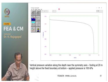
And this is our pressure distribution along the entral axis along the sorry this is sorry this is the surface settlement bowl and this is the the vertical pressure variation along the Symmetry plane symmetry axis.
