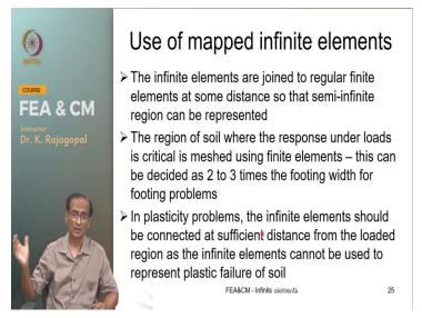
See the use of the mapped infinite elements is very simple the infinite elements are joined to regular finite elements at some distance so, that our semi infinite nature of the soil can be represented. And the reason of the soil where the response under the loads is critical is missed using the finite elements. Normally or the predominant influence of any applied load on the surface is felt up to some 2 to 3 times the footing diameter or say even 5 times the footing size.
