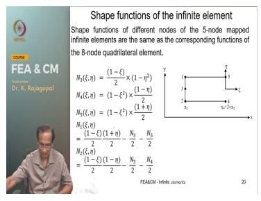
So, now let us look at the shape functions for the infinite elements and the infinite element of considered only 5 nodes out of the 8 nodes and the other 3 nodes are at infinite distance.
