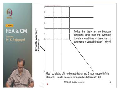
And we can do the same thing by connecting infinite elements at different distances. So, in this case the infinite elements are connected at 1.5 times the fitting width and when we use finite elements we should be careful about the boundary conditions. So, on both the sides we have supported the vertical surface on smooth rollers whereas at the bottom surface both x and y direction displacements are constrained by connecting hinges to all these nodes.
