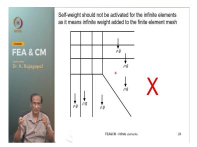
And the other precaution is we should not activate any self weight on the infinite elements. It is also very important because these infinite elements they represent infinite volume and your loading on the infinite elements means you will have tremendous loads in the load vector.
