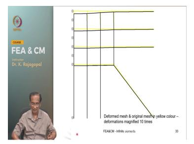
And this is our deformed mesh when we connect the infinite elements at 1.5 times the footing width.
