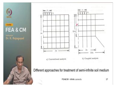
So, here we have 2 meshes one is a purely a conventional mesh with finite elements whereas the other one is called as a coupled analysis where you have some finite elements or where you have a region with finite elements and then another reason with infinite elements. And let us say that we connect the infinite elements at a distance of beta times or the radius, radius of the footing or half width of the footing.
