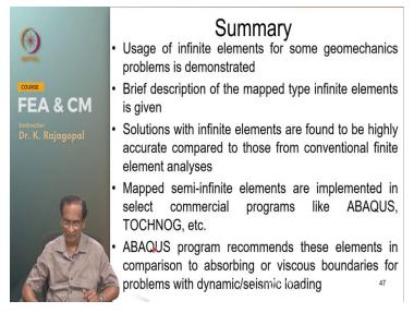
So, just to summarize the use of infinite elements for some geomechanics problems is demonstrated we have seen for footing problems circular footing and then the wall footing or a strip footing and then we have seen for pile foundations. And the mapped infinite elements are very similar to our isoparametric elements except that they have singularity in their mapping functions.
