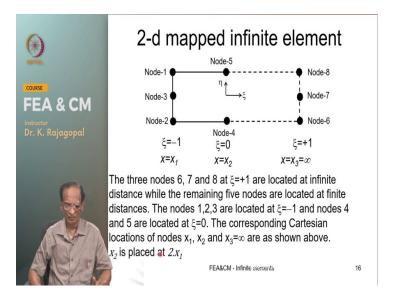
And we can imagine this map infinite element in 2 dimensions and then write our shape functions and mapping functions. So, let us let us look at see our mapping functions in the desired Direction they are developed in terms of the singularity at Xi of + 1. So, our M 1 is - 2 Xi by 1 - Xi and M 2 is 1 + Xi by 1 - Xi. Then in the eta direction our along this line there are 3 nodes.
