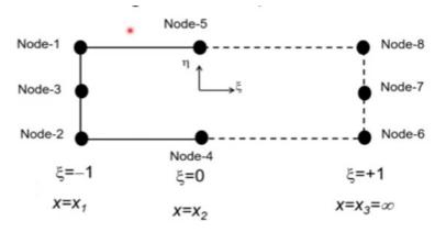
1, 2, 3 or at Xi f - 1 and nodes 4 and 5 are at Xi of 0 and the nodes 6 7 8 are at Xi of + 1 and the Xi of - 1 refers to x 1 Xi of 0 refers to x to and usually x 2 is taken as 2 times x 1. (Refer Slide Time: 25:37)
