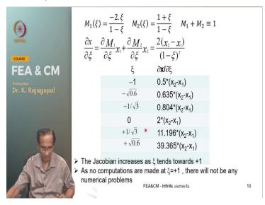
And our M 1 is - 2 Xi by 1 - Xi and M 2 is 1 + Xi by 1 - Xi and if we sum up these 2 mapping functions we get exactly one and M 1 + M 2 of 1 means there is a unique mapping unique mapping between the Cartesian space and then the isoparametric space. And so, and then at Xi of + 1 we have infinite distance and let us calculate the dou x by dou Xi that is our Jacobian determinant for the one dimensional problems.
