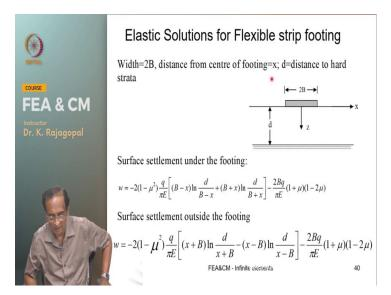
And we can verify our results even for strip footing and the solution for a strip footing are given in terms of the depth to the hard strata. So, let us say that the D is the depth to the hard stratum and this is our equation for settlements W within the for a point within the footing and the settlement equation for a point surface point outside the footing.
