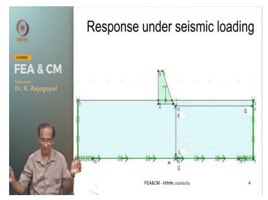
And just to illustrate I have a small problem like let us say we have a dam and that is resting on the soil and then we are giving some seismic excitation and there are some moving boundaries or viscous boundaries. And let us monitor the deformations at this point a very close to the dam.
