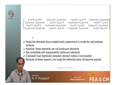
And once you go through this orthogonal transmission and this is your stiffness Matrix and the global coordinates. And these nodal link elements they have enabled early researchers to model the slip between the surfaces between the concrete and the steel or between any masonry blocks and so on. But these nodal link elements there is these are not continuum these are at particular points at the nodal points.
