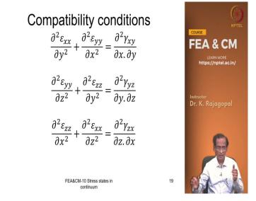
We can also write this compatibility equations in terms of the strains Epsilon xx and Epsilon yy and Gamma xy it is actually remember that our gamma xy is defined in xy plane and xy plane means we have two displacement components u and v right and along the x axis we have the Epsilon x x and along the y axis we have Epsilon yy.
