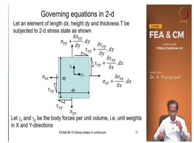
So, let us look at a two dimensional stress state because more easy to imagine and let us consider an element having a length of dx and the height of dy and in the outer plate direction let it have a thickness of t and it is subjected to some a two dimensional stress State Sigma x and then on the left hand side and the sigma xx plus some other quantity on the right hand
