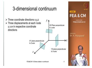
And now let us move on to more complicated materials like our structures like our continuum and in general a continuum could be in three dimensions. So, we define three coordinate axis x, y and z and then we have three displacements u along the x axis V along the y axis and then w along the z axis. And we can also as we draw these three axis we can also imagine three different planes say y z x z and then xy planes like this.
