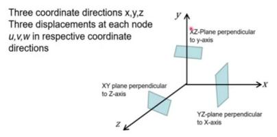
Like perpendicular to x axis we have the y z plane and perpendicular to y axis we have this xz plane and then perpendicular to z axis we have our xy plane and because we need these planes to be able to imagine our stresses and the strains.
