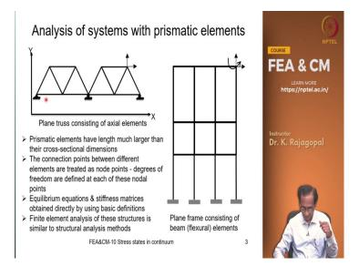
So, till now we were looking at only the prismatic elements which are long compared much longer compared to their cross-sectional area and we have seen different type of structures like the plane trusses and the plane frames and so on. And the advantage that we had is that we can readily identify all these connection points where the different members are joining and we can treat them as nodes.
