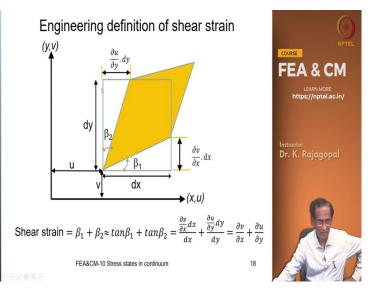
Let us look at what is this shear strain let us take a rectangular element like this and we twist it out of shape. So, that there are some angles beta1 and beta2 and our Shear strain we can write as beta 1 plus beta2.
