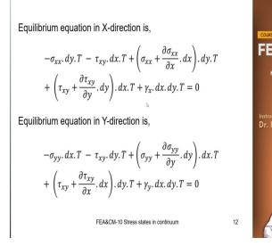
And so, we can write all these quantities and this unit Force sorry I think it should be gamma x but it got mixed up. So, gamma x and Gamma y these are basically our unit weights in x direction y direction these are the body forces per unit volume.
