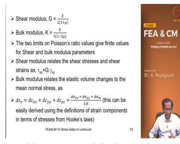
We can define two modulus parameters one is the shear modulus G as E by two times one plus mu and bulk modulus K is E by 3 times 1 minus 2 mu. And the two limits are the Poisson's ratio we can imagine that is minus one to plus 0.5 if you look at these two relations the shear modulus and the bulk modulus. So, if your mu is exactly equal to minus 1 or more than minus one you will have a problem because you will your shear modulus is negative.
