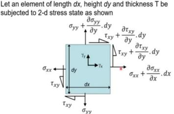
Let  $\gamma_x$  and  $\gamma_y$  be the body forces per unit volume, i.e. unit weights in X and Y-directions
