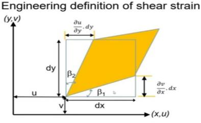
And since we are that is our basic definition or the definition of Shear strain is the change in the right angle. And since we are dealing with the small deformations beta1 can be approximated as tan beta1 and beta2 can be approximated as tan beta2.
