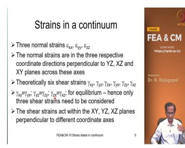
And the strains within a continuum we could have a different type of strains. So, we can have three normal strains Epsilon xx Epsilon yy Epsilon zz.
