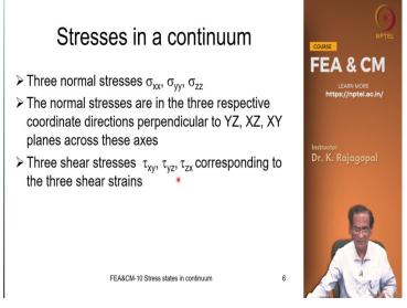
And then corresponding to these strains we will have stresses we have three normal stresses Sigma xx Sigma yy Sigma zz and these are along the three coordinate axis x, y and z normal to some planes as indicated earlier and then we will also have three Shear stresses Tau xy Tau yz Tau zx and the normal stresses that normal to some planes whereas the shear stresses that act along the plane like xy yz and zx and so on.
