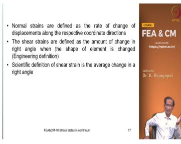
So, the normal strains are defined as the rate of change of displacements along the respective coordinate directions. So, Epsilon xx is a dou u by dou x and Epsilon y y is a dou v by dou y Epsilon zz is dou w by dou z the rate of change of displacement along the three respective coordinates. On the other hand our shear strain is defined as the amount of change in the right angle. So, when we twist some element out of shape the change in the right angle.
