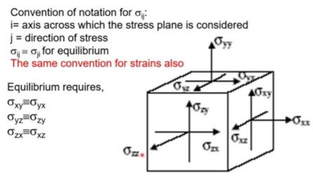
Like for example if you are looking at along the x axis we have the yz plane. And so, whatever stress that you are considering is acting a normal stress is acting across that particular plane and the j the second subscript j refers to the direction of stress and this Sigma ij is identical equal to Sigma ji for our equilibrium purpose. Because so, Sigma xy is equal to Sigma yx and is actually sometimes I use the Tau for shear stress sometimes Sigma xy but just bear with me.
