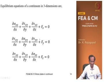
So, in general for three dimensional case we can write like this along the x axis.
