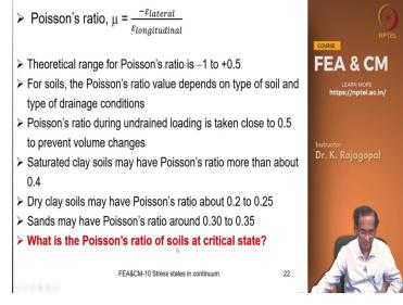
And how do we define the Poisson's ratio this is how we define minus of Epsilon lateral divided by Epsilon longitudinal the minus sign is to indicate or to take care of the the change in the sign. So, if you apply tension in one direction the other direction we have compression or if you apply compression in one direction in the other direction there is elongation. And our Poisson's ratio is a positive quantity cannot be negative.
