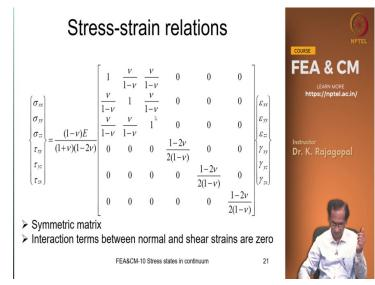
And by inverting these relations we can get our sigma in terms of the strain like this Sigma xx Sigma yy Sigma z Tau xy Tau y z Tau zx is is this product multiplied by this Matrix and then we have the six strain components Epsilon xx Epsilon yy Epsilon zz gamma xy gamma yz gamma zx and if you notice we have a symmetric constitute to matrix. See the same thing we have seen even with this the constituted Matrix for bar element and beam element actually.
