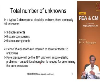
And before that let us look at how many unknowns we have to solve for. See we have totally 15 unknowns unknowns in any three dimensional problem we have three displacements we have six strain components then we have six stress components. So, we have totally 15 unknowns. So, we need at least 15 equations to solve for these 15 unknowns but then we have one more extra unknown because we are dealing with the geotechnical problem. So, we should not forget about our pore pressures.
