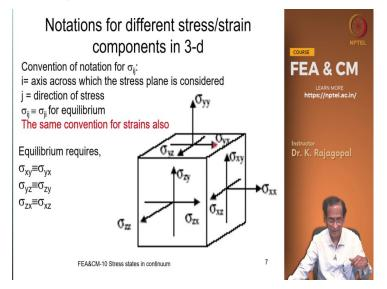
So, pictorially this is what we can see we have three coordinate axis x, y and z and these are the positive directions and we can imagine the right hand side the screw for all our sign conventions. And the convention in elasticity is to denote all these quantities with two subscripts and sigma ij like our Sigma xx Sigma xy and so on. And i and j they refer to two different things i is the axis across which the stress plane is considered.
