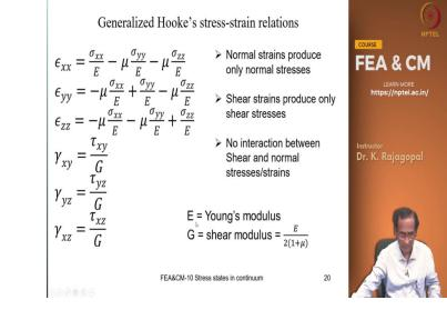
And we need some relation between the stress and strain. So, that if you know the strain we can calculate stress or if you know the stress we can calculate the strain and for this we go back to generalized hooks loss that were given to us in I think in the 1700's 1772 or something like that our Epsilon xx is Sigma xx by E minus mu times Sigma yy by E minus mu times Sigma zz by e.
