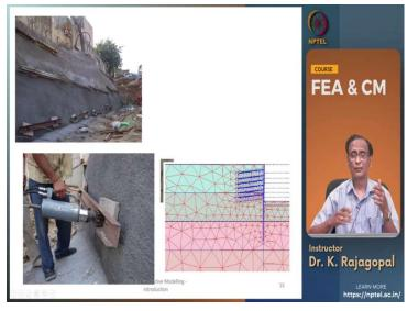
So, here you see and the surface itself is protected by spray concrete and then some rows of these nails they are pre-stressed and. So, how do we model this? See in the finite element analysis is very simple you see here you have your slope either a vertical slope or an inclined slope. Then we have these nails that are installed at different depths and then we gradually excavate the soil.
