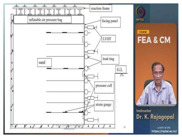
And the soil was subjected to failure by applying uniform pressure through an inflatable air pressure bag.
