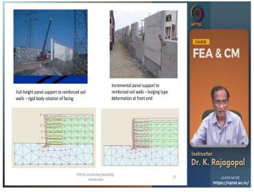
And here is a I am showing two different types of retaining walls one is called as a full height panel wall where the entire height of the wall is made up of only one single concrete panel and it is a manner of deformation is going to deform like a rigid body. Is going to rotate around the bottom it is like this and this is the upper picture is the actual picture taken from the site whereas this is the bottom one is from our finite element analysis.
