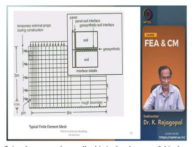
And this is the finite element mesh actually this is the close-up of this the problem that we have here is the facing panels are made of one material these are hard materials and then the soil is there and then we have the reinforcement geosynthetic reinforcement. And each one has its own stiffness. The soil is the weakest among all these three materials and at the junction between these different materials what do we do?
