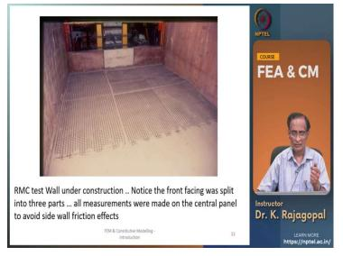
Let us say we can apply this finite element analysis for analysis of retaining walls. Here you see one test retaining wall this was built at Raw Elementary College of Canada and this is about three meters high wall and this was an experimental wall that was in fact I was part of this research work long time back. And we were interested in knowing what will be the failure mechanism.
