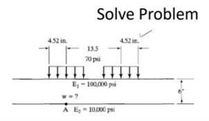
Figure 2.20 shows a set of dual tires, each having contact radius 4.52 in. (115 mm) and contact pressure 70 psi (483 kPa). The center-to-center spacing of the dual is 13.5 in. (343 mm). Layer 1 has thickness 6 in. (152 mm) and elastic modulus 100,000 psi (690 MPa); layer 2 has elastic modulus 10,000 psi (69 MPa). Determine the vertical deflection at point A, which is on the interface beneath the center of one loaded area.
