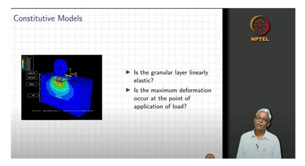
The granular layer is also not going to be elastic it is pressure dependent confinement pressure dependent and the point of application of the maximum deformation is also there is going to be a slight offset here.
