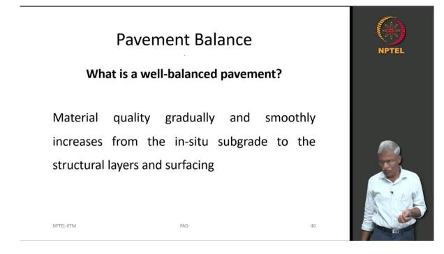
Now comes the next concept which in my opinion is a very important concept, what is called as a well-balanced pavement. Here, the material quality gradually and smoothly increases from the in-situ subgrade to the structural layer and surfacing. That means, you do not give a drastic jump in the modulus value as you go from the subgrade all the way up to the surface material. So, this is what is called a well-balanced pavement. (Refer Slide Time: 26:21)
