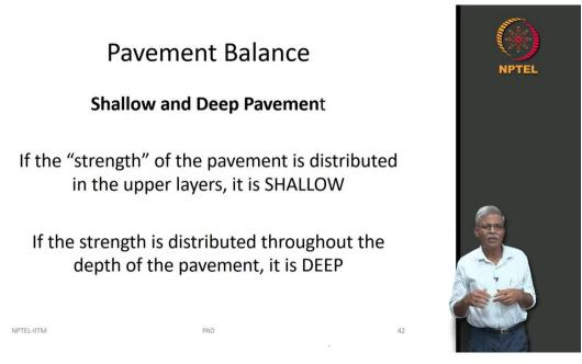
Then there is also a concept of shallow pavement and deep pavement similar to shallow and deep foundations. If the strength of the pavement is distributed in the upper layer, it is called shallow pavement, and if it is distributed throughout the depth, it is called deep pavement. Again as part of an exercise, you may want to also relate a balanced pavement with shallow pavement as well as with deep pavement.
