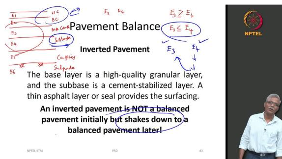
In an inverted pavement, you can have a base layer which is a high-quality granular layer but your subbase could be a cement stabilized layer. This is your wearing course, binder course, base course, subbase, capping layer and subgrade. The modulus values are  $E_1$ ,  $E_2$ ,  $E_3$ ,  $E_4$ ,  $E_5$ ,  $E_6$ . Now let us take a look at these two  $E_3$  and  $E_4$ . Now  $E_3$  can be greater than or equal to  $E_4$  or  $E_3$  can be less than or equal to  $E_5$ .
