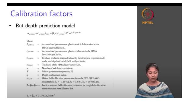
So, let us take a rut depth equation model which is given in MEPDG. So, this is the rut depth prediction model.
