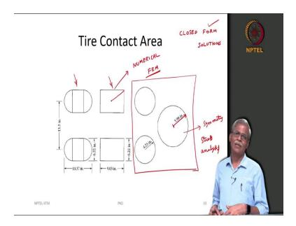
Now, we can have different types of tire contact area. The correct way of doing it will be this you could also do it this way, but what we are going to do is in this way. Why? Because there is a symmetry here our life becomes very easy when we are going to do the stress analysis part because, since there is a symmetry here all I really need to do is to compute the stresses and strain across one radial direction and this whole thing can be computed.
