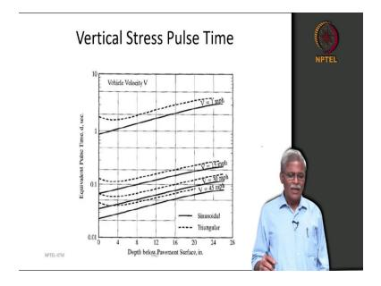
And, interestingly as you go down in the depth at various layers below the surface of the pavement, you are going to see the time duration that you see here is going to be increased. Because as you go down the pavement the load contact area you can see the pressure bulb
