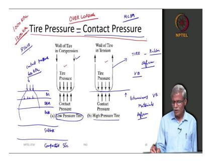
Now, comes the most important concept and the most important assumption that we are going to make as far as pavement engineering is concerned bituminous pavement engineering is concerned. Now, we you all know what exactly the tire is made of. The tire is typically made of rubber.
