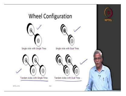
So, to just give you a brief perspective about this thing is single axle with single tire, single axle with dual tire, tandem axle with single tire, tandem axle with dual tire. Of course, you can also have tandem axle with single tire and in fact, next time after you listen to this video and when you just go watch in the road and focus your attention on the axle configuration, you will see that there are some Indian trucks that will also have a tandem axle with a single tire.
