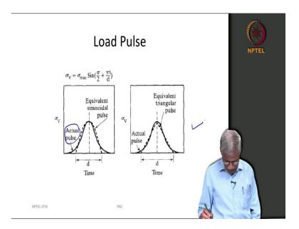
So, this is what is the waveform here. And, in fact, the actual pulse is going to be something like this. You could write it in terms of equivalent sinusoidal pulse or equivalent triangular pulse.
