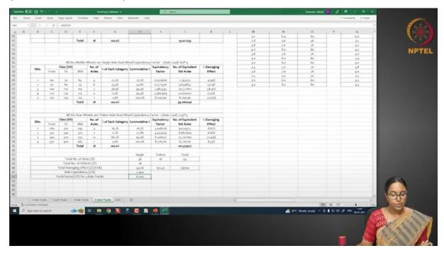
Likewise, all the damaging effects are summed together and divided by the number of vehicles to get a truck factor of 8.70. So, for all the 4 truck categories we have determined the truck factor separately.
