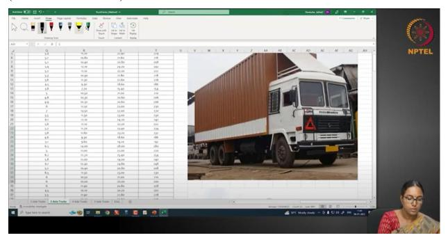
We will move on to the next one which is a 3 axle truck. As you see here in this picture, there is a front axle with single axle single wheel and at the rear there is a tandem axle. But for convenience it is written as 2 axles. Altogether, there are 3 axles. This is why this class is named as 3 axle truck.
