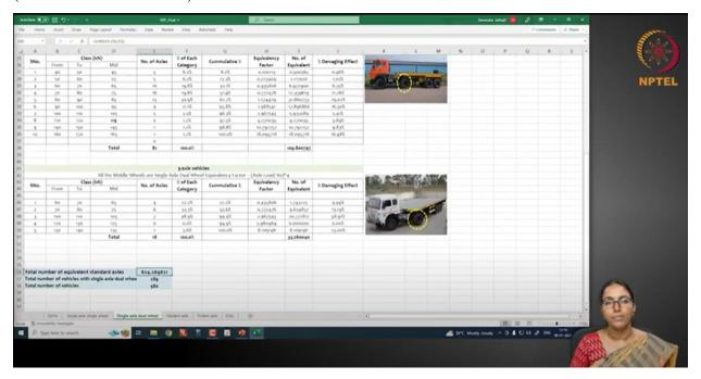
You see that this is from the first type of vehicle, this is from the second type of vehicle and this is from the third type of vehicle, all common type of axles with a standard axle load of 80 kN. Now, using the same approach, you find the equivalent axle loads, you sum up together. So you get the total equivalent single axle loads due to this axle type.
