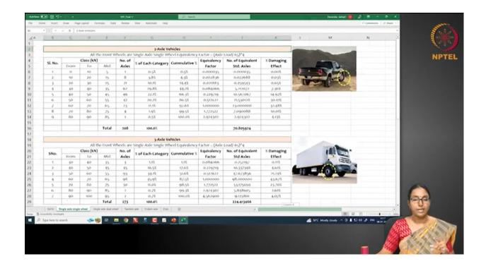
You can put the axles in different class categories, the frequency can be measured. And then we can calculate the equivalency factor for this particular class of truck using the standard load. So, multiply the number of axles with the equivalency factor to get the total equivalent standard axles. So, from the first class of vehicle, you got 70, the second class of vehicles is 224, third class of vehicles is 75 and the fourth class of vehicles it is 19.
