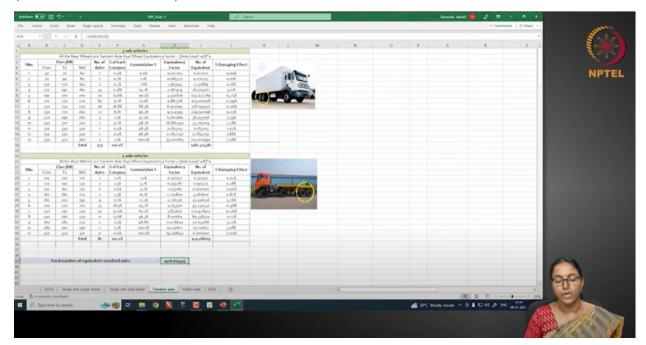
Now, moving on to the tandem axle, you had like 2 vehicle classes where there were tandem axles. Find the total equivalent standard axles for those classes.
