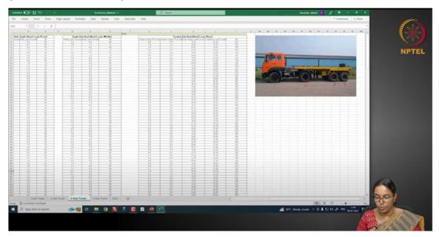
The next truck category is a 4 axle truck. First of all you have data for the single axle single wheel, and then you have data for the single axle dual wheel, then tandem axle. So, equivalency factor can be obtained for the first one using a standard axle load of 65 kN, the second one with a standard axle load of 80 kN and the third which is a tandem axle, with a standard load of 148 kN.
