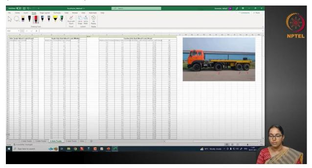
And then you have a 4 axle truck here, you see that at the front there is a single axle single wheel assembly and then you have a single axle dual wheel assembly and then there is a tandem axle which is counted as 3 and 4. So, there are 2 axles. Altogether there are 4 axles. So, this class of vehicle is classified as a 4 axle truck.
