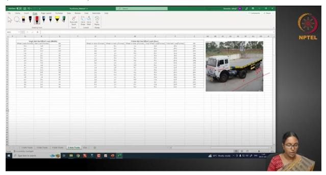
And then comes the 5 axle truck. You see here that there is a front axle which is single axle single wheel and there is a single axle dual wheel which is your axle number 2 and there is a tridem axle with dual wheels. So, altogether there are 5 axles. This class of truck is named as 5 axle for convenience. So accordingly, I have all these axle sheets here.
