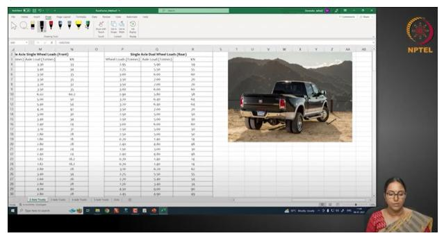
Once the data is collected, you can see that in this excel sheet I have marked it as different pages. One is the 2 axle truck, the other is named as 3 axle truck, 4 axle truck, then 5 axle truck and so on. So, if you see there is a 2 axle truck, this is an example of the 2 axle truck that you are considering. There is a front axle with a single axle single wheel and a rear axle with a single axle dual wheel. This class is categorized as a 2 axle truck in the study.
