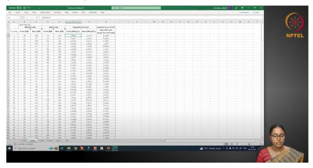
Now similarly for the second category of vehicles, you see that this is 3 axle truck. So, equivalency factor for the front axle and the rear axle (tandem axle) is calculated. The total equivalent standard axles or truck factor for each one of the trucks is calculated.
