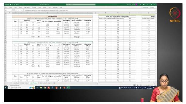
The data is divided into different axles, and then the damaging effects for each one of them are calculated as before.
