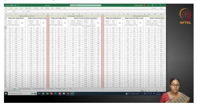
As we have already seen, there were like 4 classes of vehicles which were named as 2 axle vehicle, 3 axle vehicle, 4 axle vehicle and 5 axle vehicle for convenience. So, this is the data for 4 classes of vehicles. Compile all the single axle single wheel loads together. From all the 4 categories, single axle single wheel will be put together and you determine the equivalent standard axle loads from that category of axle.
