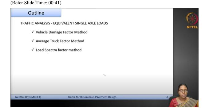
So, the outline of this session will be, you will see how the traffic is analyzed in terms of equivalent single axle loads by three different approaches. The first one is a vehicle damage factor method, the second is an average truck factor method and the third is a load spectra factor method.
