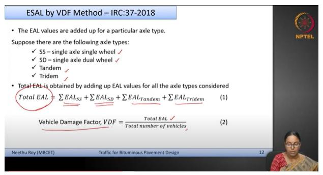
So for a particular axle type, you have different axle load groups you add all the equivalent axle load values together to get the total ESAL corresponding to that axle group.
