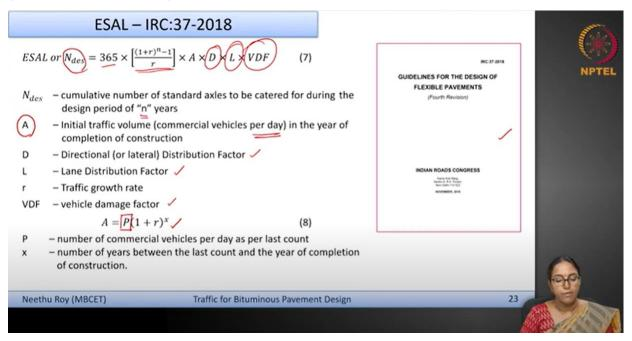
Now let us see based on using all these input parameters how the total design traffic is considered. You call it as  $N_{design}$  or the equivalent single axle loads ESALs.
