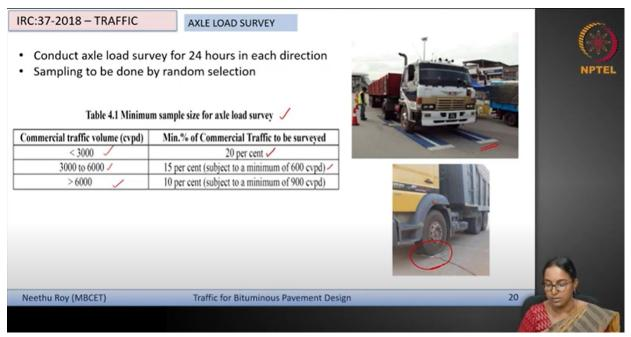
Now as per IRC: 37-2018 it suggests that you have to conduct the axle load survey for 24 hours in each direction of traffic. Now it may not be possible to stop all the vehicles in a particular stream and measure the traffic loads.
