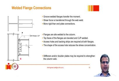
So, here you can see a typical rigid connection in this diagram wherein the beam flanges are directly welded to the column. So, as we have discussed the beam flanges are group welded and they are meant to transfer the design moment capacity design moment demands and the shear force is transferred through the web. So, the web could be welded to the column but also it is quite common to bolt it to the column.
