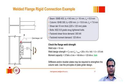
Now these welds of course they are given as con complete joint penetration welds and they are done on both flanges. So, the thickness of the weld or the throat size of this weld will be 16 millimeters that is the thickness of the flange of the beam. So, we will use 16 millimeters as the throat size and using that we can calculate the capacity of this weld under tension. So, now let us calculate the strength of these welds under this type of loading wherein this flange undergoes tension.
