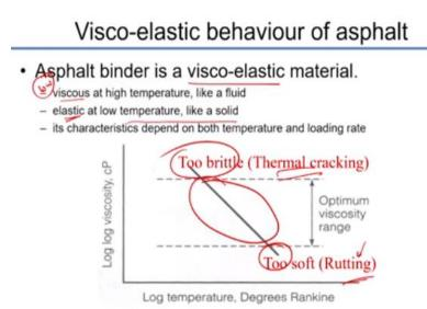
Most important with asphalt, it is highly dependent upon the temperature; the application of the asphalt is highly dependent upon the temperature, because asphalt is a viscoelastic material. Remember in the chapter on polymers we talked about the fact that one of the important consideration of polymers is to assess its viscoelastic behavior and the range of temperature over which you can get satisfactory performances as a solid.
