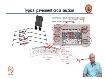
What is this pavement cross section? As I said flexible pavement is the system of layers that are acting together. And the load intensity keeps reducing as we come from the top layer to the subgrade. So, how is this happening? What are these layers? So, if you look at the simplest arrangement which is shown here. The bottom most layer is obviously the soil or subgrade. On top of which we are sometimes having a sub base which is a compacted and stabilized soil.
