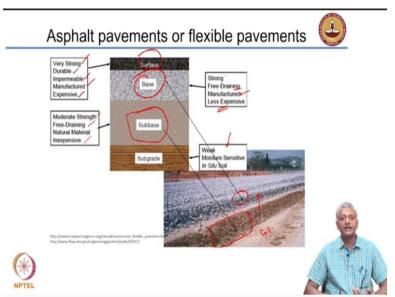
Again a picture-based scenario is depicted here. So, as I said you have the soil here. This is the soil, on top of the soil, you have the sub base. The soil itself may be weak and moisture sensitive or it may be strong, we do not know. You have to determine the quality of the soil first before you decide on the number of layers and thickness of each layer that is required. So that is all part of pavement design which you learn later in your high way material course.
