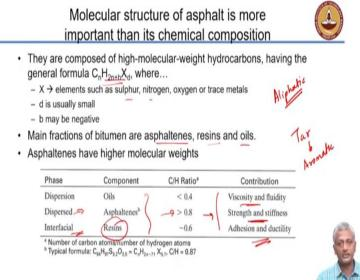
So again, coming back to the structural asphalt, as I said it is a long chain hydrocarbon or aliphatic hydro-carbon, not aromatic but aliphatic hydrocarbon. And this is where it differs from tar, tar is aromatic. So if you remember your organic chemistry, aromatic means it has got the benzene rings in it whereas asphalt has a long chain structure. This is a general formula of asphalt. You can have elements like Sulphur, nitrogen, oxygen or trace metals in the structure of the hydrocarbon itself.
