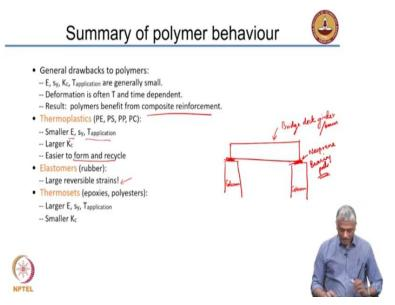
So just to summarize, polymer behavior as we said compared to metals and ceramics or concrete, the general drawbacks are that the modulus of elasticity, the temperature of application, the fracture toughness, these are generally small. Deformation is temperature and time dependent. Very important to remember that. And again, sometimes you can improve the characteristics by composite reinforcement. What do you mean by that?
