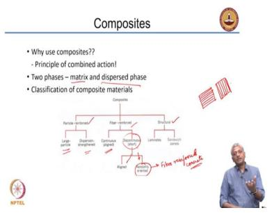
So we talked about polymers and let's take a look at how we can make these polymers a lot more versatile for engineering applications by making them into composite materials. First of all why do we want to use composites? Simplest example is reinforced concrete. Why are we using the composite because concrete is good in compression and steel is good in tension. We combine the good characteristics of both and give a composite that produces a synergistic effect. So that's a combined action.
