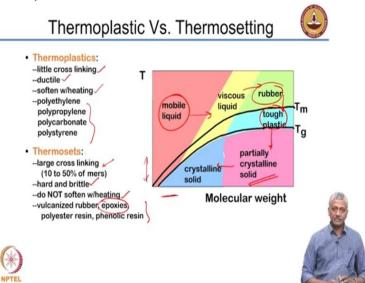
Again thermoplastic versus thermosetting, what is being shown here is that how does the molecular weight of the materials affect the way that it responds to temperature. If you make a polymer with a very high molecular weight consisting of very large number of chains, you will have to significantly increase the temperature to cause it to change its behavior. So that's what is being shown here.
