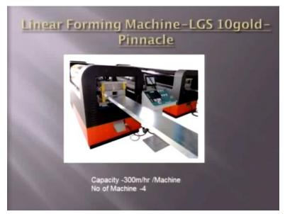
And what we see here is called a rolling machine; now, the rolling is the one which makes all these structural sections.
