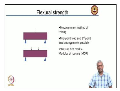
The other way of testing the strength indirectly is flexure or bending. In most cases, the tension becomes our problem and contradicts bending like in a beam; for instance, when we bend the beam, the bottom fiber of the concrete is under tension, which is where it causes cracking. That is what exactly we do in this case of flexural strength determination. We have this beam which is simply supported.
