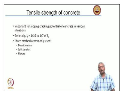
What about tensile strength? We always talk about compressive strength because that is what concrete is good at. But still, for some applications, we need to measure the tensile strength of the concrete. How do we measure tensile strength? We have to prepare a concrete and then pull it apart and measure the load at which the failure occurs. The problem with this, which we call direct tension, is that it is tough to hold the concrete.
