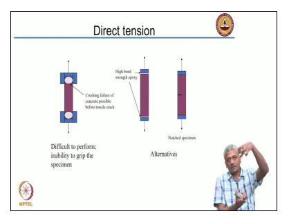
So what is direct tension? As I said, direct tension means we are simply holding the concrete and pulling it apart? However, if the concrete specimen is large, the amount of pressure that we need to put to hold it together at the ends may sometimes cause the crushing of the concrete at the ends. Our concrete at the ends may crush because we are putting too much pressure to hold the specimen.
