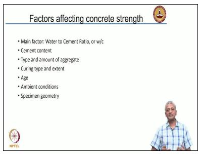
So once the concrete sets and hardens, it starts gaining strength. Concrete starts gaining strength rapidly at first, and then the rate of strength gain slows down. Usually, as in concrete design, we are familiar with concrete strength at 28 days. We generally talk about 28-day strength. So in most cases, we will see that concrete is specified in terms of a grade we specify.
