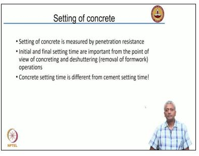
We talked earlier about the fact that cement hydrates by reacting with water and slowly leads to the setting and hardening of the cement itself. Now please remember that concrete is a conglomerate that is made with cement, water, and aggregate. So what happens is how the concrete sets are not the same as the way the cement sets. Please remember that in cement, we talked about using this test called the Vicat test to determine the setting time of the cement.
