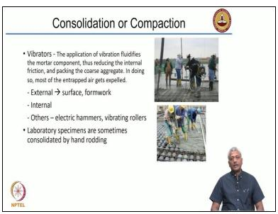
So you place the concrete down, next step is to compact it. Because you have a reinforced concrete structure, when you are pouring the concrete, this concrete may not properly go around the reinforcement and properly encapsulate it. To ensure that happens properly, you
