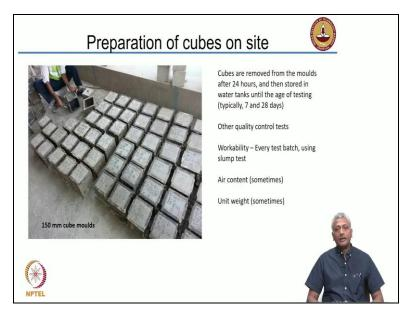
Now on the job site as I said there has to be some quality control done to ensure that the concrete that is supplied is meeting the demands of what the design has been done for. As I said one of the common tests that is done the job site is the slump test, to determine the workability. But apart from the slump test, you also need to ensure that you determine the strength somehow.
