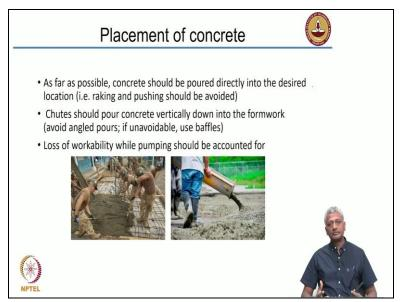
So, after you have conveyed the concrete you are going to be putting it in the form work or placing it. So, as far as possible concrete should be poured directly into the desired location. You do not want to pour it at one end and then start raking it. So here, for example, you see a picture of these workmen, so concrete is getting discharged here and these people are actually pulling it.
