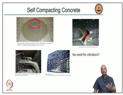
So, as I was saying, you need to design structures with concretes that have high flow ability. So, that they need very little vibration or almost no vibration as in the case of self-compacting concrete. So here this is a slump test that has been done with self-compacting concrete. As you can see the concrete is simply flowing out. There is no slumping here, it is actually totally flowing out almost like water.
