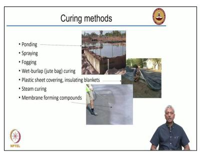
Now there are different ways in which you can do this. For horizontal members like this, you can simply create an embankment and store water on top, which is called ponding. Sometimes you may just spray water using a water spray or a pipe. Sometimes you can fog the environment by using very fine sprays of the water which creates more or less like a mist around the concrete.
