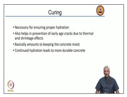
After finishing is done, the next step is curing. Curing is absolutely necessary for ensuring a proper hydration of the cement. So you put in cement, water, stone and sand into the concrete, the cement and water is having a certain level of proportion that is in such a way that the water is required for reacting with the cement and producing this hardened concrete structure. If this water starts evaporating even before the cement fully reacts, then it is not going to be good for your concrete.
