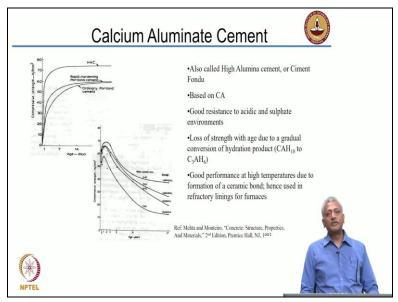
There is also a cement called calcium Aluminate cement where the raw materials are not the calcium carbonate limestone and clay, but limestone and bauxite that is aluminum oxide. So these produce compounds that are rich in calcium oxide and aluminum oxide or calcium aluminate. These are calcium Aluminate cements also called high alumina cement.
