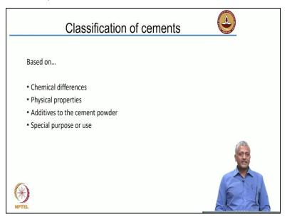
Let us look at how cement can be classified; they sometimes are used in different applications. I already told you the example of using cement in a column in a high raised building versus using the same cement in a dam. We need different characteristics for the applications. Because of that, we sometimes have to define cement of different types which can be employed for specific applications.
