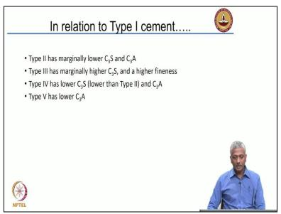
So in relation to type I cement that is general purpose cement, type II will have marginally lower  $C_3S$ , and  $C_3A$  type III will have marginally higher  $C_3S$  and a higher fineness. Type IV will have a lower  $C_3S$  and also lower  $C_3A$  content and generally much higher  $C_2S$  content. Type V will have a lower  $C_3A$  content; that is what we see in this table regarding the quantities of the compounds present in different types of cement.
