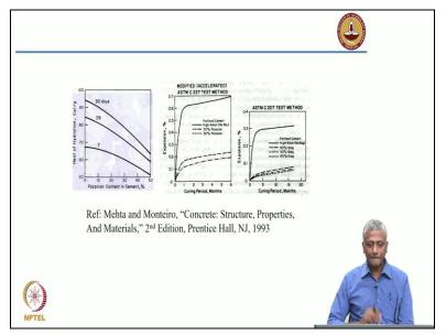
Again, this shows us the heat of hydration in calories per gram with respect to the pozzolanic content in the cement at seven days; it is coming down a little bit at 90 days the extent of reduction of the heat of hydration is significant. In some instances where we have problems of undue expansions of the concrete, pozzolanic materials bring down the expansion and reduce the tendency for cracking.
