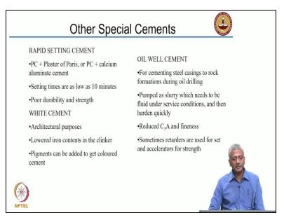
There are other special types of cement also which are used for very specific purposes like **rapid setting cement** is generally consisting of some amount of plaster of Paris which is calcium sulphate hemihydrate or sometimes it may have Portland cement plus calcium aluminum cement so that as soon as we mix with water within a short period of time let us say as low as 10 minutes, we get a rapid stiffening.
