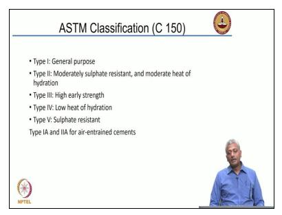
We are going with this universally applied classification called ASTM or American Society For Testing and Materials ASTM. It brings out standards and all kinds of materials and processes and test methods and so on. So the ASTM classification for cement is included in ASTM C 150.
