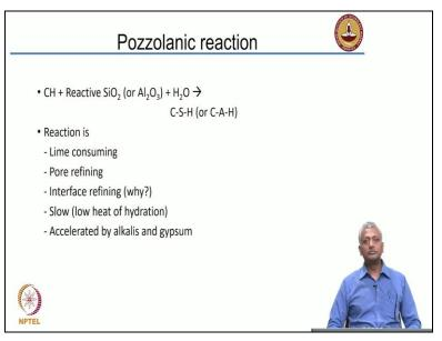
Again, the pozzolanic reaction is the reaction between calcium hydroxide that forms from cement hydration and reactive silica that we get from the pozzolanic material to produce additional calcium silicate hydrate. So what we are doing is we are consuming this lime, we are refining our porosity, and we are also refining the interfaces. So if we consider aggregates, the cement paste around the aggregate is getting a lot denser in the case of a pozzolanic reaction.
