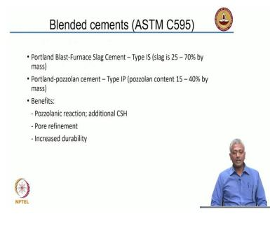
In some cases, we blend certain components to enhance the cement's properties or lower the cost. So there are different types of blended cements that are permissible as per the ASTM standards. One is called Portland blast furnace slag cement called type Is, and the slag is nearly 25 to 70% by mass in the cement. Now, what is this blast furnace slag?
