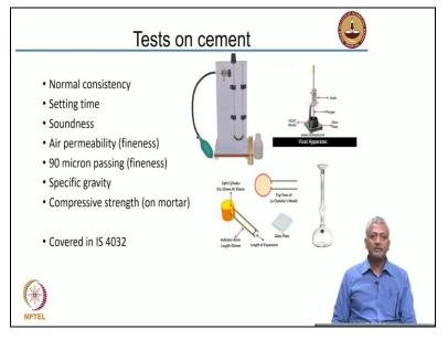
I was talking previously about tests and cement. I am just showing the same here the normal consistency and the setting time are done with the Vicat apparatus, shown here. So we have a mould into which we mix our cement paste and put it inside; then we have a plunger of one centimeter, which is made to rest on the top of the cement paste and then dropped, and this plunger plunges into the cement paste.
