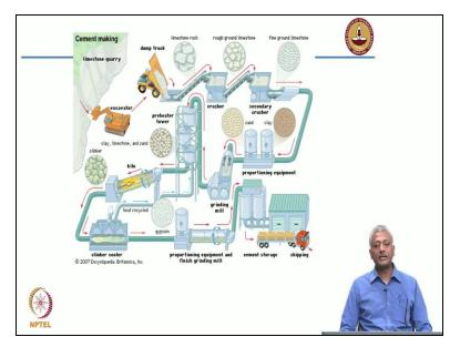
So this is a schematic that describes our Portland cement production process. So we have our quarry from which limestone is getting extracted; after extraction, it goes through some crushing, we have a primary crusher, secondary crusher, and so on. Finally, we get fine grounded limestone and get it stored in silos.
