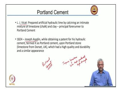
So what is cement? We discussed this in the stone, brick, and mortar chapter cement are nothing but binding material. It reacts with water and sets and hardens. Lime does the same thing; however, lime reacts with water; pure lime reacts with water to convert into calcium hydroxide and absorbs carbon dioxide from the atmosphere to convert to calcium carbonate and harden.
