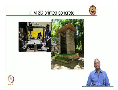
At IIT Madras, we have done a fair bit of 3D printing ourselves, and we have constructed this India's first 3d printed structure; this is just a very small room, but the idea was to print something of the size of a toilet. Subsequently, we printed a toilet and are in the process of printing actually a full-scale house that will be available on the campus of IIT Madras. I would welcome all of you to come and see the house that we printed entirely with 3D printed components.
