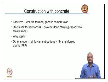
So now, one essential fact with concrete, as it is true with other construction materials like stone or brick concrete, is fragile in tension. So it is used primarily for compression-related applications that means wherever it can bear compressive loads, it is happy. Nevertheless, as soon as we get tension into concrete, it starts cracking. So concrete is weak in tension and good in compression, and because of this, we usually combine concrete with steel.
