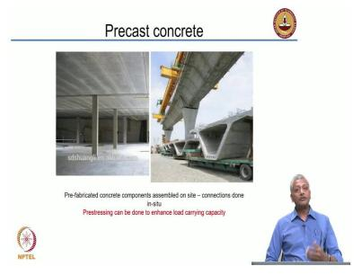
And of course, today, we cannot escape an urban setting without the use of precast concrete. Concrete is prefabricated and brought from factories and assembled on-site, just like what we do with steel construction. Especially with the construction of segmental bridges, what is done is each segment is cast in a factory and is brought to site and assembled on site.
