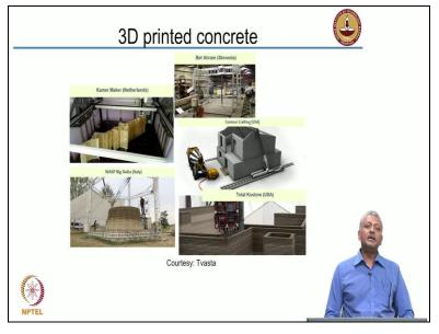
Of course, in the most modern of developments, people are talking about printing concrete now. I showed a picture earlier where the formwork had to be put in place. We need to define the shape of the concrete and then put the reinforcement and then place the concrete into it in a more or less liquid form. But what if we can print the concrete in the shape of the structure that we want, and that is what is being done with 3D printing.
