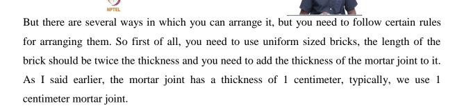
So we want to get uniform lap uniform bonding between bricks, as a result of which we need to satisfy this rule that the length of the brick should be twice the thickness plus the thickness of the mortar joint. So does this meet our needs, for example, if you consider a modular brick, as I said, it should be 19 \* 9 \* 9, if you do not consider the thickness of the mortar joint. So this 19, obviously, is equal to (2 times 9) + 1.
