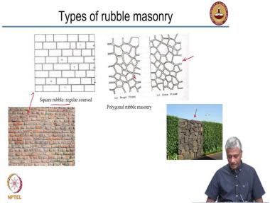
Now, this is something you would have probably seen in several locations, is called polygonal rubble masonry, where you have rubble of different shapes, which is arranged in a
