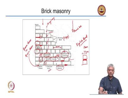
Now, again, just to bring to light the use of toothing, or steps, this is exactly the picture that I was talking about. So when you provide steps like this, after the end of the day's work, you can continue the next day's work by arranging bricks and blocks on this side. And this kind of a feature is called toothing. You are leaving behind gaps, which are unfilled so that you can continue the next day's work filling up those gaps. That is called as toothing.
