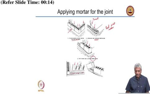
Let us now take a look at how mortar is typically applied for a joint. So let us take this scenario for a wall that has been constructed from the ground level up, that means from a foundation that is in the base of the ground and then from there we are constructing the wall up. So first what is done is that the blocks are placed without the mortar on the foundation. So here, it is a strip foundation.
