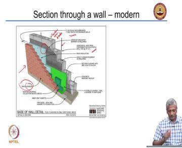
In a modern building, we utilize the engineering concepts optimally. So, what are these engineering concepts that we are trying to utilize? One aspect is aesthetics. in this wall, the outer surface looks like a brick wall and we call it a brick veneer or a brick facing. Essentially, it's the outer surface which is simply giving it a nice aesthetic brick like appearance, but the actual wall itself is made with concrete blocks. These are hollow concrete blocks.
