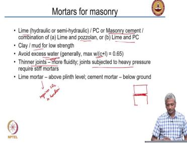
Coming back to the use of different types of materials for mortar, what type of mortars are typically designed for masonry and how should we actually use this? As I said, the materials typically are lime, Portland cement. Sometimes in some countries, we may also have special cements called masonry cements. In India also masonry cement was available in the past. Today it is not available. Today only plain cement is available, which has to be mixed with sand.
