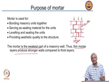
Why is mortar needed? Of course mortar is needed to bond the masonry units together because it keeps everything in place. It serves as a seating material for the units. Units sit on it and make a level surface for the course. Mortar is also nice to break the monotony of the
