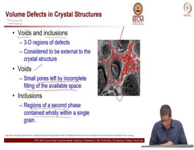
Now let us go into the fourth type of defect which is volume defect. We started with point defect, then we talked about line defect, then we talked about you know the surface or plane defect, that is a grain boundaries and then we are now going to talk about volume defect which are mainly voids and inclusions. Void means air void, there is no material present.
