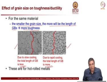
So, because of this, the size of the grain boundary has an influence on the toughness, we can say that. Now here when you look at the left side micrograph, it is like you know this is 100 micron, the length of this little draw straight line is about 100 microns. So, you can say the size of this, let us say 0.8 millimeter is the distance from this point to this. So, you are looking at within a millimeter in size.
