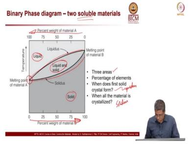
Now binary phase diagram for 2 soluble materials, this is one of the simplest phase diagram which we are going to discuss here. You can see here again this is the composition, here you can see the same thing for material A at the top axis and then material B at the bottom axis. Now that means if I draw a line along this, I have 25% material B and 75% material A is the composition.
