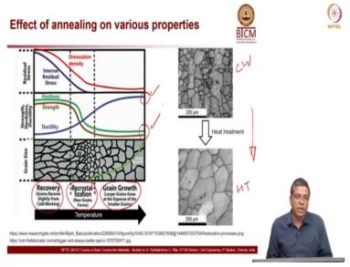
Now generally when we look at this, you can see that heat treatment generally tends to increase the grain size from the cold work stage. So, this is cold working stage and then this is after the heat treatment. Now look at the graph on the left side you can see recover, so this
