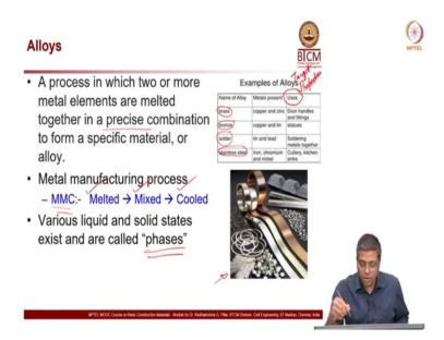
Now let us talk about alloys. What is alloying? It is a process in which 2 or more metal elements are melted together in a precise combination, so not just mixing but in a very precise combination to form a specific material with certain target properties. Now there could be properties like it should be malleable, like you know the ability to flat and then it could be you need to have an increased strength.
