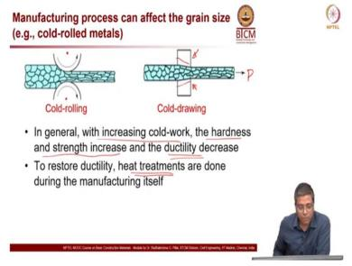
Or cold drawing also, this is the 2 difference in a major way by which we do cold working, there is a common term, cold working or strain hardening etc. So, cold rolling where you have 2 rollers here and the material is coming out in a through these rollers, whereas in case of cold drawing, you are actually pulling the metal through a die which is probably, this is a die and then you can see the change in the dimension or reduction in the dimension as the material is pulled through that.
