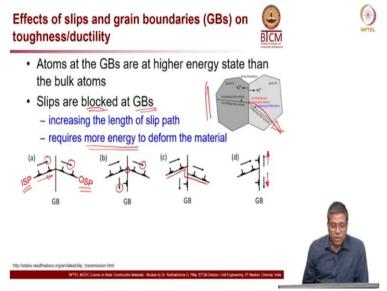
Now effects of slips and grain boundaries or I am going to call grain boundary as GB here on toughness and ductility. Now atoms at the grain boundaries are at higher energy state, when we talk about atoms which are at the grain boundaries, they are at higher energy state than a particular atom within the grain boundary. Now slips are blocked at grain boundaries, so we just to show that drawing earlier, same drawing I have repeated here.
