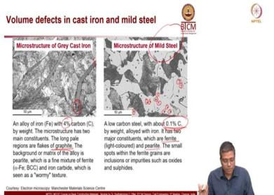
Now these are some real examples, the first picture is a microstructure of grey cast iron. You can see in the cast iron you have a lot of these flakes present. You can see this is another flake and in this picture, you have 3 big flakes of graphite present, you can see here graphite, so this is an image of an alloy of iron and 4% carbon. So, cast iron has a lot of this carbon present, 3 to 4% easily by weight.
