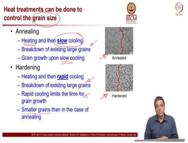
Now heat treatment, what is the idea? When you do this heat treatment, it changes the grain size to a desired level as you want. So, 2 major way of heat treatment which I am going to discuss here briefly are annealing and hardening. So, in case of annealing, what we do is we heat the material and then allow it to cool in a slow manner, heating and then slow cooling and in case of hardening, it is heating but cooling is very rapid.
