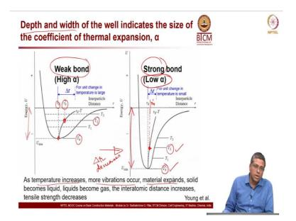
Now, how, let us look at how the shape of this diagram, or what does it mean when it, or how it is related to the thermal expansion, coefficient of thermal expansion. Or how we can use these graphs to understand the coefficient of thermal expansion. So, let us look at the case of a weak bond, weakly bonded material on the left side. There, I put high alpha. That means, high coefficient of thermal expansion.
