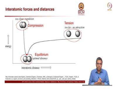
Now, let us get into a little bit on the interatomic forces and the distance between atoms. And how they behave when you apply a force in compression and in tension. So, that is what we are going to look at. So, it is a typical Condon-Morse diagram. I will show it in the next slide. So, you can see it here. This case is two atoms in equilibrium. They are not necessarily touching each other, but they are at an optimal distance between them.
