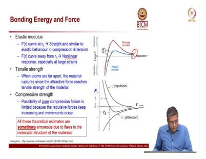
So, here you can see. On the top right sketch, very clearly, the dF/dr which we are talking. So, the slope of that. In the red curve, which is a strongly bonded material, the slope is higher. That means, when you try to pull, there will be much force acting against the pulling force. The blue one is a weakly bonded thing. That means, when you try to pull, the force generated is still going to be not that high as in the case of the red one.
