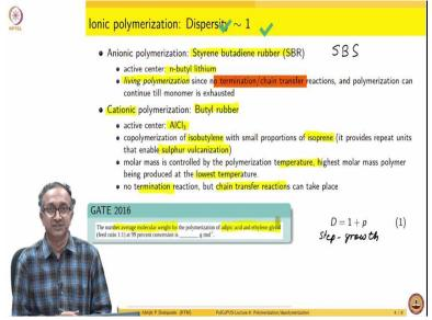
So, we will just look at ionic polymerization before we start looking at new ways of thinking about polymerization. The advantage of ionic polymerization is that dispersity which is the ratio of weight average molar mass to number average molar mass can be close to 1, 1.05, 1.07,1.1. Such polydispersity indices are possible when we use ionic polymerization and this is
