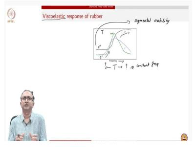
So, in the closing what we will do is look at a generic response of rubber materials given that they are used so much in case of these damping applications and energy dissipation applications. So, viscoelastic response of rubber generically is follows. What we have is if we subject the material to low frequencies since the material is in the rubbery state segmental mobility is there and segments can fluctuate.
