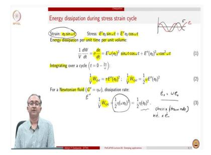
So, let us start by first thinking about energy dissipation. Since a lot of dynamic testing involves an oscillatory test. So, we will consider energy dissipation during a cycle of test. So, as we have seen several time that what we do during a cyclic test is maybe apply a let us say sinusoidal stress or we could apply sinusoidal strain and then we basically measure what happens to the strain as a function of time.
