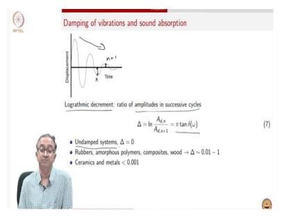
So, let us look at and consider what is the phenomena happening during damping of a material. So, damping is basically where we put the material and let us say one side is vibrating the other side should not feel it. So, for example a machine which is located on a floor we put vibration isolation pads below so that when the machine vibrates, we on the floor should not get feel the vibrations.
