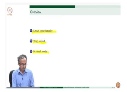
And in this lecture, we will first spend some time looking at linear system response while discussing the viscoelastic response and then the two model which are examples of linear models which means that they are applicable for only small deformations and so we will look at the response of these two models to a creep and stress relaxation.
