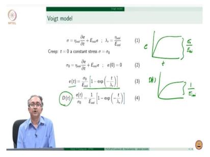
So, let us look at Voigt model which is one of the simpler models of viscoelasticity. So, if we ignore the term which is the derivative of strain then basically, we have stress proportional to strain. So therefore, that just an elastic response which is like a Hookean solid response. On the other hand, if we ignore the second term then this response is nothing but what is the response for Newtonian fluid where stress is proportional to strain rate.
