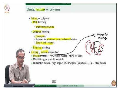
So, blends are basically mixtures of polymers. And both of these polymers can exist themselves as, homopolymers as single polymers, where we mix them in required proportions to optimize or to tune properties. And this mixing can be done by 2 ways, we can do melt blending, where we take both of the polymers or if it is a blend of 3 polymers and take all 3 polymers to the melting temperature and above and then we can do the mixing.
