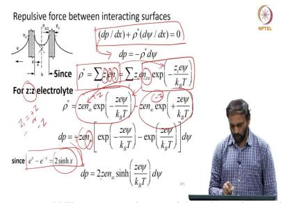
So, therefore now we would like to express the potential you know the so, what we will do is we will again do some simplifications. So, that is the force balance and therefore I can write recast this as dp = - rho star multiplied by d psi and we know that the charge density in solution can be written as summation i  $z_i$  e times  $n_i$ . So, all that we are doing is we are summing up the charge contribution because of different types of ions in solution.
