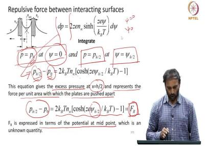
I could integrate this and use the boundary condition that at a in the so, when we consider that the potential is at a very large separation at a very large distance from the surface we know that the potential would be 0 that is size equal to 0 and at that location we say that the osmotic pressure which is proportional to the concentration of ions that you have at that location is  $p_0$ . And at h / 2 the potential is psi h / 2 and correspondingly the osmotic pressure p is p at h / 2.
