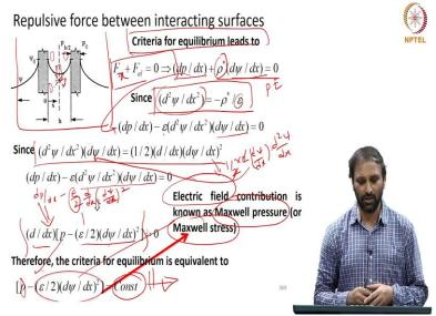
So, therefore the criteria for the equilibrium is  $F_x + F_{el} = \overline{0}$ . Therefore dp / dx + rho star times d psi / dx = 0 and we know this from the Poisson equation; the Poisson equation 1 dimension is d square psi / d x square = - rho star / epsilon. So, I can instead of rho star I can replace so, that is the dp / dx term instead of rho star I can replace that with epsilon times d psi / dx and d square psi / dx square times d psi / dx.
