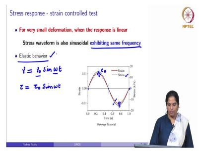
So for any elastic behaviour when we subject the material to a sinusoidal strain the red colour one is a strain waveform. So, we have given an input for this strain amplitude which we defined it as  $\gamma_o$ , strain amplitude. And it is a sinusoidal waveform so if we want to mathematically represent this training sinusoidal waveform we can write it as  $\gamma$  to be  $\gamma_o \sin \omega_t$  it is a sine waveform with amplitude to be  $\gamma_o$  and the frequency as  $\omega$ .
