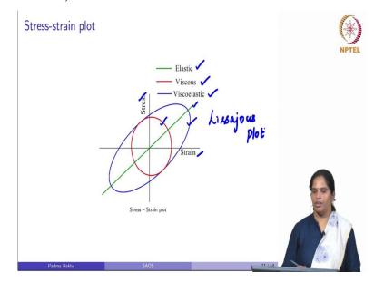
So, this will be an ideally stress strain plot for a different material elastic, viscous and viscoelastic material for a sinusoidal shearing. So, stress strain plot for a elastic material is straight line for a viscous material is perfect circle as a phase angle is 90 degree and for a viscoelastic material it is elliptical. We call this viscoelastic material as stress strain plot and there oscillatory shearing as a lissajous plot.
