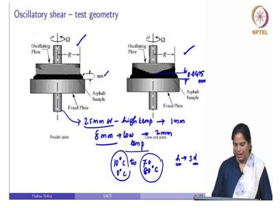
So, oscillatory shearing as we said is it is nothing but a shear flow in inducing a shear flow in a material. So, in an oscillatory shear we keep a material between the two plates maybe a parallel plate as shown in this figure here or between a plate and a cone system and we keep the bottom plate fixed and the top plate oscillate or in case both plate oscillating in a different directions. So, by doing this we are subjecting the material kept between a two plate to a shear flow.
