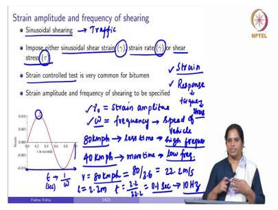
So, by oscillating the top plate we are subjecting the material to a sinusoidal shearing. So, you can control the speed and the deflection of an oscillation so that we will get a controlled sinusoidal shear strain are controlled sinusoidal shear rate are controlled shear stress. So, we control the oscillation in such a way that the material is subjected to a sinusoidal strain or a sinusoidal shear rate or sinusoidal shear stress.
