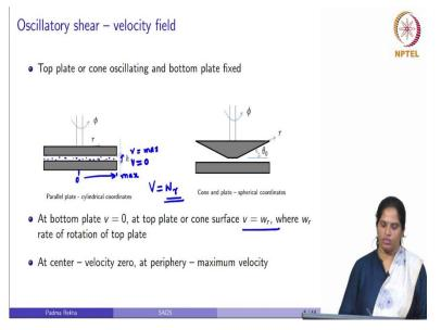
So, in an oscillator a sheared system we keep a sample between two plate and oscillate so while doing this the particle between a two plate is not subjected to a uniform motion. So, if a bottom plate is stationary and the top plate is rotating, so the motion of a particle sticking to the bottom plate will be 0 and the velocity here will be 0 at the bottom plate. So, if the top plate is oscillating
