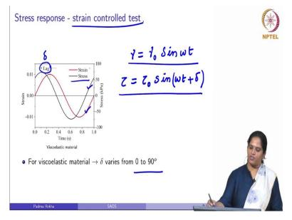
So, you for a sinusoidal strain control test if the material exhibits a viscoelastic behaviour we also get a sinusoidal stress with the same frequency but the lag value here then that is a time lag between peak stress and a peak strain will lie between 0 and 90 degree. So, this is the basic concepts which we are going to use to define a material functions. So, let us write the equation for a strain and stress, so control a strain and can be written as  $\gamma_o \sin\omega t$  sinusoidal strain.
