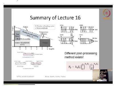
So, this is more or less the clear way in which I will put together the summary of the lecture. So, one need to very clearly understand, if you look at the top left picture, the strain versus the number of cycle, fatigue is always at the center, which means the load application that you give will result in strains that are substantially less, and the number of cycles will be more and there is a linear viscoelastic regime that we will see at the starting point.
