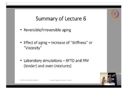
So, the effect of aging can in essence lead to increase in the stiffness or viscosity of the material and laboratory simulations exercise for RTFO as well as PAV and oven mixtures where detail here.
