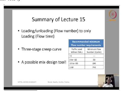
So, what is the most important way in which you will say, a flow number test is where you load it and unloaded, whereas in the flow time test you just only apply a load. The basic model that is
