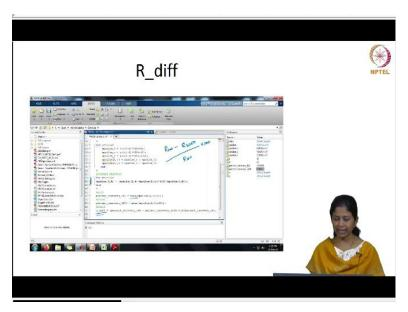
And we are also required to calculate R difference which is percentage recovery at 100 minus percentage recovery at 3200 divided by percentage recovery at 100 which is nothing but R100 minus R3200 divided by R100 into 100. So, this is R difference. So, this you can straight away calculate because these are 2 numbers. So, you can specify it in the same manner, you have to note that here we are giving it as a loop because we have to calculate this individually for all the 20 columns.
