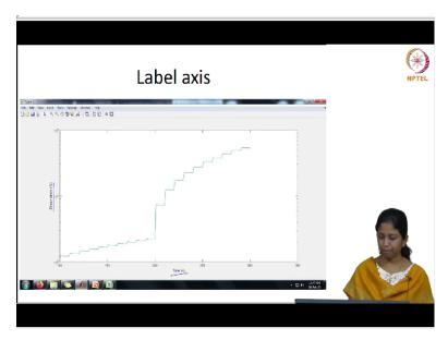
So, then we will be able to see that the axis labels are also now generated. So, it is a plot of time versus shear strain right. So, this is how we make plots using the data. Next, we start calculating some parameters using this particular data. So, the 2 parameters which we are going to see here are percentage recovery and non-recoverable creep compliance.
