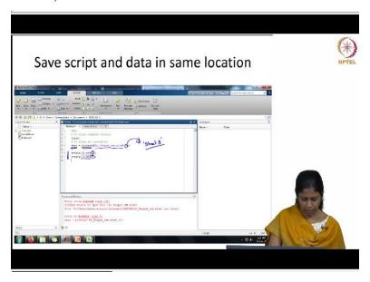
So, what you do here is, we write a code right, this data is a variable. This data can be anything x y, p, q whatever it is. So this is a variable right. So, this data is equal to xls read, to read an excel file, we have to specify it as xls read, you provide the file name exactly within a single quote. This is very, very important, you have to specify the name of the file with extension. So this is AS Unaged 1mm.
