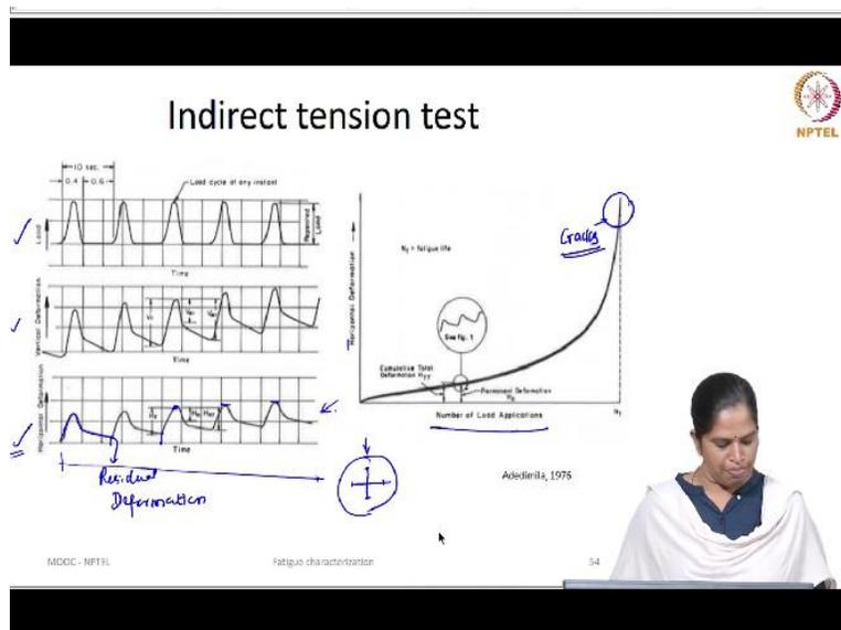
This what we apply it and this is what the response you get it. If you measure only the horizontal deformation, this is a load you apply and this is a horizontal deformation you get. In case if you fix a 2 strain gauzes like this, you apply a load here, you have horizontal strain gauge as well as a vertical strain gauge, you will get 2 deformation one is horizontal deformation and other one vertical deformations.
