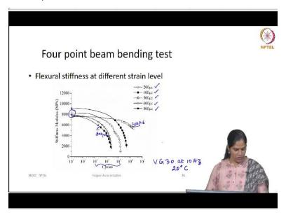
So, you can see a flexural stiffness calculated for different strain levels for this is for refer time bituminous mixture prepared with VG 30 sample at 10 hertz frequency when tested at 10 hertz frequency and 20 degrees Celsius. So, the test was conducted at 200, 400, 500, 600, and 800 micro strain. So, you can see that the refer time fitness modulus decreases with the loading and you have to note that this is a logarithmic scale.
