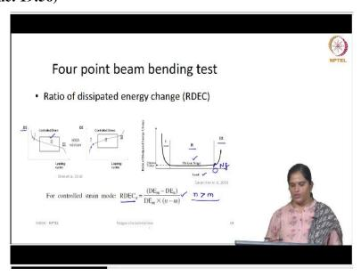
So, this is again a hypothesis what we mean. So, in the next method we use the energy dissipation ratio for calculating the fatigue life. So, as we said already in a strain control test, the
