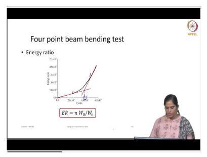
So, this energy dissipation ratio when you look into the trend of energy ratio, you will see energy dissipation trend exhibiting a two stage slope, one is a refer time where the slope is very small, second is as the slope increases. So, this 2 stage slope the point of intercept of this 2 stage slow this determined as a number of cycles to failure. So, this is the energy ratio method.
