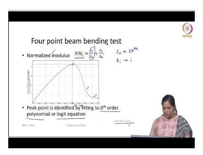
And ASTM D8237 recommends a normalized modulus for calculating the fatigue life. The normalized modulus is nothing but the normalized value of stiffness modulus where Si is measured at the initial cycle, that is at 50th cycle and So is at the 50th cycle which is at the initial cycle Si is at the i<sup>th</sup> cycle. So you normalized value with respect to the initial stiffness.
