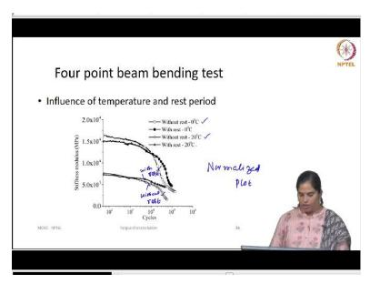
Again that the evolution of flexural stiffness also depends on the test temperature. If you see test temperature at 0 degree and 20 degree. So, this is refer time the test conducted without rest period on continuous loading at 0 degree and this is a test conducted without rest period at 20 degrees. So, 0 degree has a high flexural stiffness compared to 20 degree as expected and again the rate of decrease is also not same that you will observe when you plot a normalized plot.
