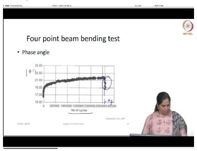
The next method of identifying or determining the fatigue life of a bituminous mixture, this using a phase angle value. So, phase angle value as the damage progresses, the phase angle is plotted as a function of number of cycles refer time, at the point of damage or the extreme point of its damage you can see the decrease in the extreme sharp decrease in the phase angle and this is taken as a fatigue life of a bituminous mixtures.
