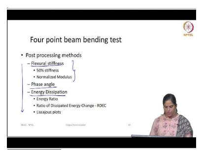
So, now we have calculated the stiffness modulus for different loads cycles. Now, we need to find out from the stiffness modulus value, we need to find out what is the fatigue life of a bituminous mixtures. There are various post processing method available to calculate the fatigue life of a bituminous mixtures. So, few of the post processing methods but not limited to this are listed here.
