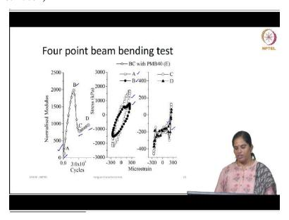
So, this is our normalized modulus curve. Now if you want to see a damage that occurs at a different stage of a normalized modulus, the damage can be seen by plotting Lissajous plot, if for an undamaged sample the Lissajous plot will be an elliptical and for as the damage progresses the Lissajous plot will be an disorient from an elliptical shape to a non elliptical shape.
