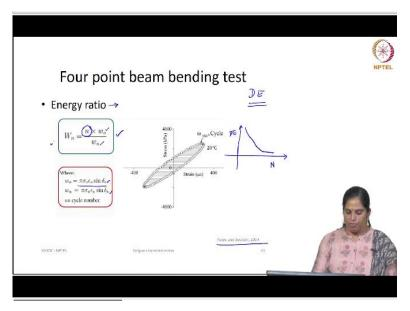
The next approach of determining the fatigue life is using an energy dissipation value, dissipated energy, which in a short form can be noted as DE. So, this dissipated energy generally, we get or we find it using an equations, we are all familiar with this dissipated energy, which is function of a stress amplitude and the strain amplitude and delta here is the phase angle, the suffix O is given for an initial cycle and the N is given for an Nth cycle.
