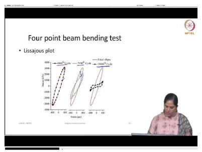
And as we said already Lissajous method in you this. So, you have Lissajous plot if the Lissajous method in this. So you have a Lissajous plot if the Lissajous plot here at the initial cycle is perfectly ellipse we assume that there is no damage in a material and as the Lissajous plot that deorient from the ellipse over as the loading cycle increases the damage occurs slowly.
