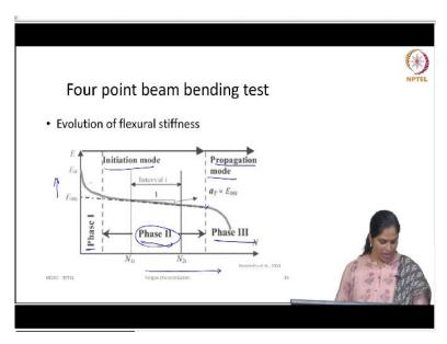
So, now we know what is flexural stiffness, but if you see the evolution of a flexural stiffness it exhibits a 3 phases. So, flexural stiffness as given in a Y axis, we have function of number of load applications, you can see a 3 phase, phase 1, phase 2 and phase 3. So, in the initial phase, there is a drastic decrease in the flexural stiffness. And in the second phase, the decrease in the value is uniform and it is gradual.
