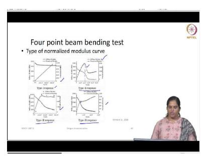
Now, if you see a normalized modulus curve as per ASTM recommendations that typically normalized modulus curve looks something like this type 2 response. So, you have normalized modulus curve type 1 type 2 type 3 type 4 response, that typically ASTM code normalized modulus curve looks like this. It increases reaches a peak value then decreases, will identify the point corresponding to the peak point as a fatigue failure point.
