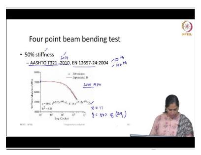
So, refer time fatigue life calculated based on the stiffness. So, then the AASHTO T321 10 now, we have 2014 revision recommends are different method of fatigue life calculations as well as per AASHTO T321 2010 and as per the EN standard fatigue life was estimated using a stiffness a value or a flexural stiffness value. It says that damage in a payment occurs when the flexural stiffness falls less than 50% of the payment.
