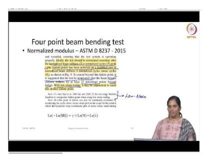
So, ASTM says that, ideally that test should be terminated sometimes or after the normalized beam stiffness and the product of normalized beam stiffness and normalized a cycle P value has the failure point that is peak value has been achieved on the graphical plot. If this is not achieved, you can use a weibull distribution as described in this note. So, this generally occurs weibull distribution conditions fitting generally occurs when we test it at very low strain level.
