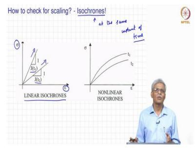
So when we do that and when we plot this particular line, you are going to see if you are going to get a straight line. The way in which it is seen here you are going to say that this is the response of the material is linear or what you really call here as linear isochrones. Now I need to make a clarification based on the statement that I made in the last lecture. In the last lecture I very clearly emphasized that one should not plot stress versus strain graph for a
