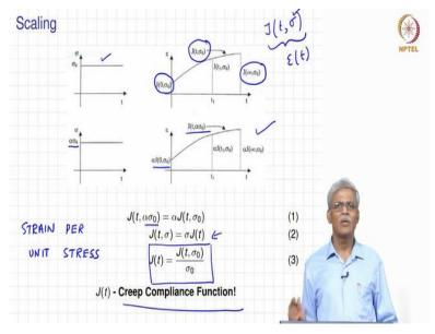
So let us keep looking at each of them as we go alone. So right now let us get back to our older definitions we defined a function called creep compliance, which had two parameters t and  $\sigma$ . So that means, for any given stress level for any given t this function returns what is called as the strain at that particular instant for any applied load given by  $\sigma$ . Right? So now let us take a look at this first picture wherein we are applying Sigma of  $\sigma_0$ .
