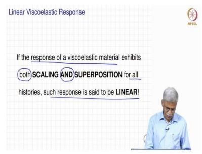
So let us make this statement very clear if the response of a viscoelastic material exhibits both this is the most important thing scaling and superposition for all stress histories such response is said to be linear. So that means when you do a creep and recovery or when you do a stress relaxation or when you test the material in frequency domain in oscillatory shear, you need to ensure that the response of the material is scalable and also superposition is valid.
