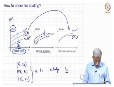
We are picking one particular time t1 and we are taking this ( $\sigma$ ,  $\epsilon$ ) pairs and trying to plot those graphs to get the check for the linearity.
