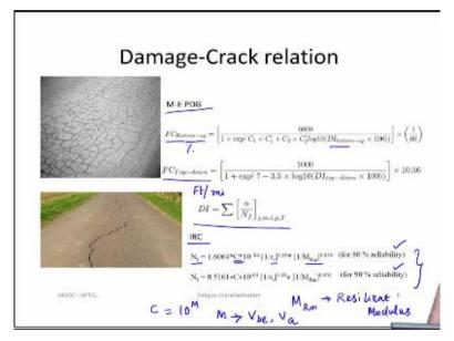
And for different truck and for different month durations and for different pavement temperature, find out what is the damage index and use this damage index in this fatigue cracking expressions to determine the extent of fatigue cracking either a top down cracking or a bottom up cracking. So, in this fatigue cracking, top down cracking is expressed in length or otherwise feet per miles.
