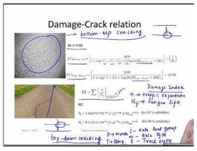
When you see a cracked or a damaged pavement, you can see a two types of crack. One is something like a group of cracks here, which we call it as an alligator crack, another is something like a longitudinal crack on the pavement. This alligator crack is said to initiate from the bottom of an asphalt layer, and we call it as bottom up cracking. So, the crack initiates from the bottom of an asphalt layer and propagates to the top something like this.
