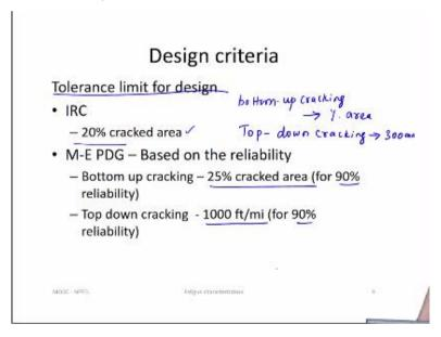
So, when do we say that the pavement has fully damaged or it cannot be used further for a traffic movement is, so there is a tolerance limit defined for the design. IRC defined the tolerance limit to be a 20% cracked area. Here, bottom up cracking and the top down cracking in terms of a units because bottom up cracking as per IRC will be something a map like crack and we do not have any issue here in defining the units for a bottom up cracking in terms of a percentage area.
