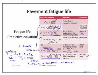
Now there are few performance prediction equations, performance prediction equation given here. When you look closer into this equation, the basic equation is of this type. Here  $N_f$  is number of repetitions to failure. So  $N_f$  value is given by a constant. It is a function of strain, 1 upon strain to the power another constant and you have an exponential equation here. So here this A and b are a regression constant and  $\varepsilon$  is a critical tensile strain in the pavement.
