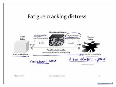
We know that the bituminous mixture in a pavement is subjected to a wide varying temperature. For example, if the pavement temperature is varying from 0 to say 70 degrees Celsius, at very high temperature, the bitumen behaves as a viscoelastic fluid like behavior and at very low temperature bitumen behaves as either an elastic or a viscoelastic solid like behavior.
