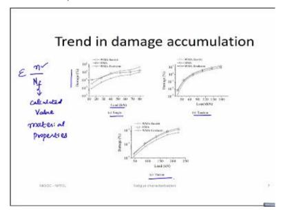
Now if you into the sample damage index of a sample, sample damage index, you can see a three picture here. One corresponds to a single axle, other corresponds to a tandem axle and the third one corresponds to a tridem axle. So now the x axis in this figure is load and y axis a damage index, which is  $^n/_{N_f}$ . So, n is actual traffic on the pavement is subjected to. This  $N_f$  is a calculated value.
