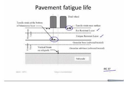
Now if you look into the critical locations, so IRC 37 gives a critical location where the crack starts. If you see this picture clearly you will have two location. One is at the bottom of a bituminous layer. You have two bituminous layers here. One is rut resistant layer another is fatigue resistance layer. If you see the tensile strain at the bottom of a bituminous layer will be critical for a fatigue damage to occur in the pavement.
